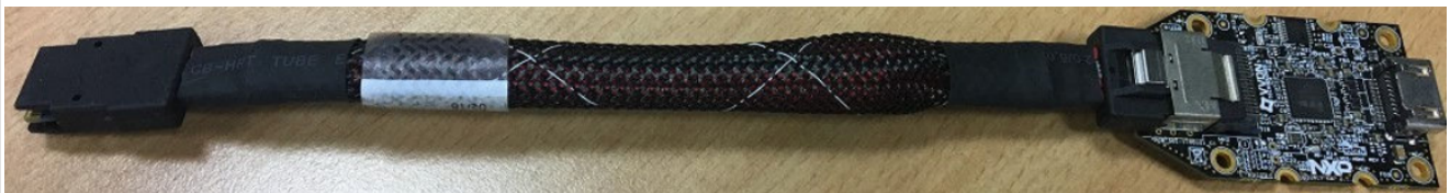
Figure 10. i.MX mini SAS cable with LVDS-to-HDMI adapter
