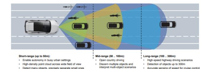
Detect many objects, precisely separate small ones next to large ones and reliably classify in real time
