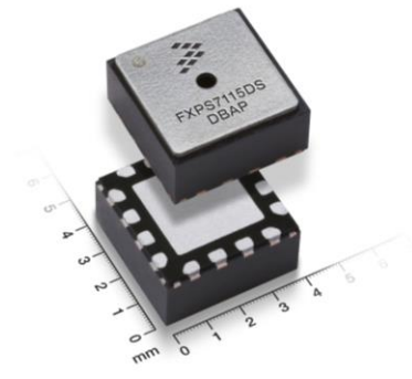
4 mm x 4 mm x 1.98 mm QFN, 16 pins, 0.8 mm pitch
