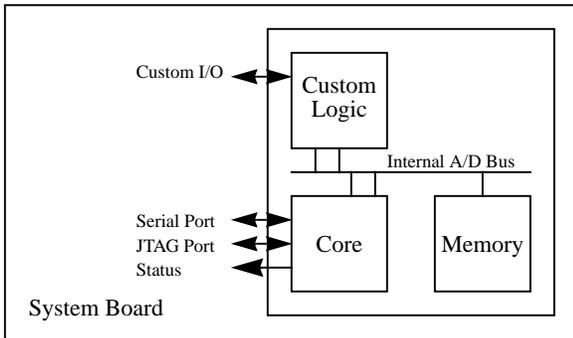
**Fig. 2** Board configuration without bus visibility
