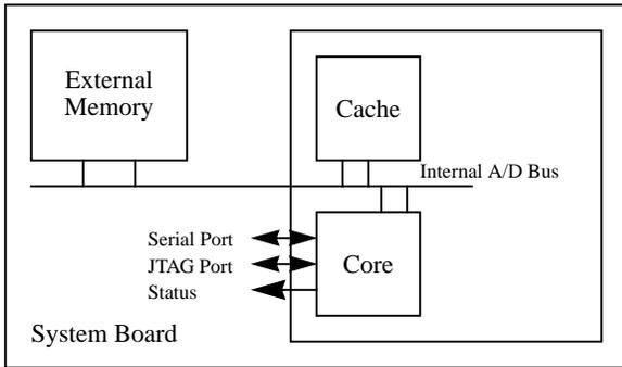
**Fig. 1** Board configuration with bus visibility
