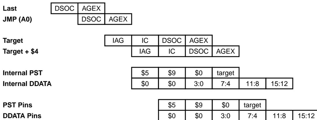
**Fig. 6** Pipeline timing example with DDATA output
