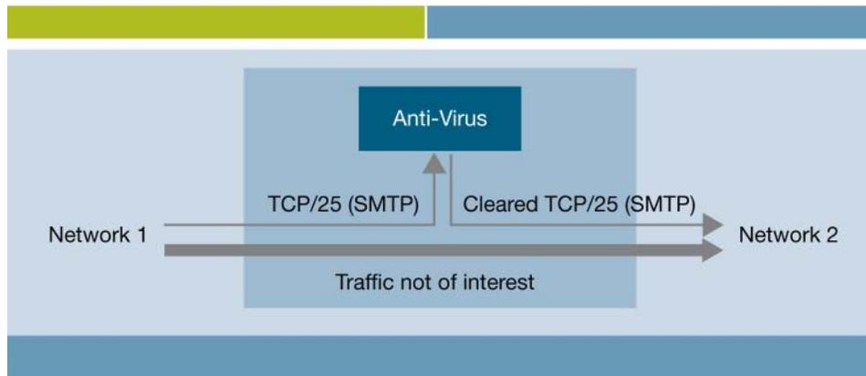
The key data path operations in a typical network AV device are as follows:
