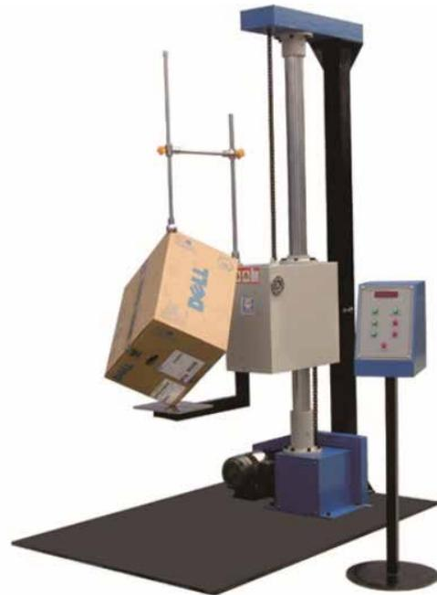
Figure 6: Drop Test Machine
