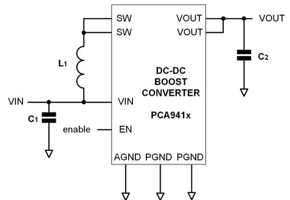
**Figure 4.** DC-DC Converter requires only three external components.
