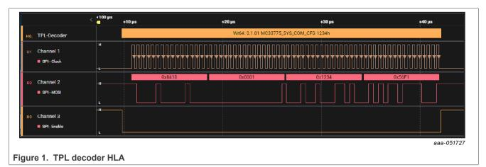
This tool is also part of the NXP battery management system (BMS) communication decoder ecosystem and can work together with the <u>KIT-TPLSNIFEVB</u> hardware board that facilitates the acquisition of electrical transport protocol link (ETPL) signals.
