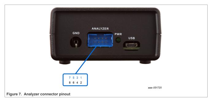
The supplied 8-pin connection cable should be plugged into the ANALYZER connector with the blue wires on top (NXP logo side) and the black wires on the bottom.
