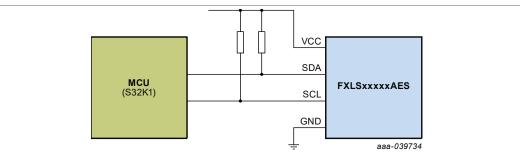
Figure 10. I<sup>2</sup>C application diagram
