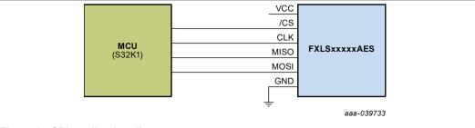
Figure 9. SPI application diagram
