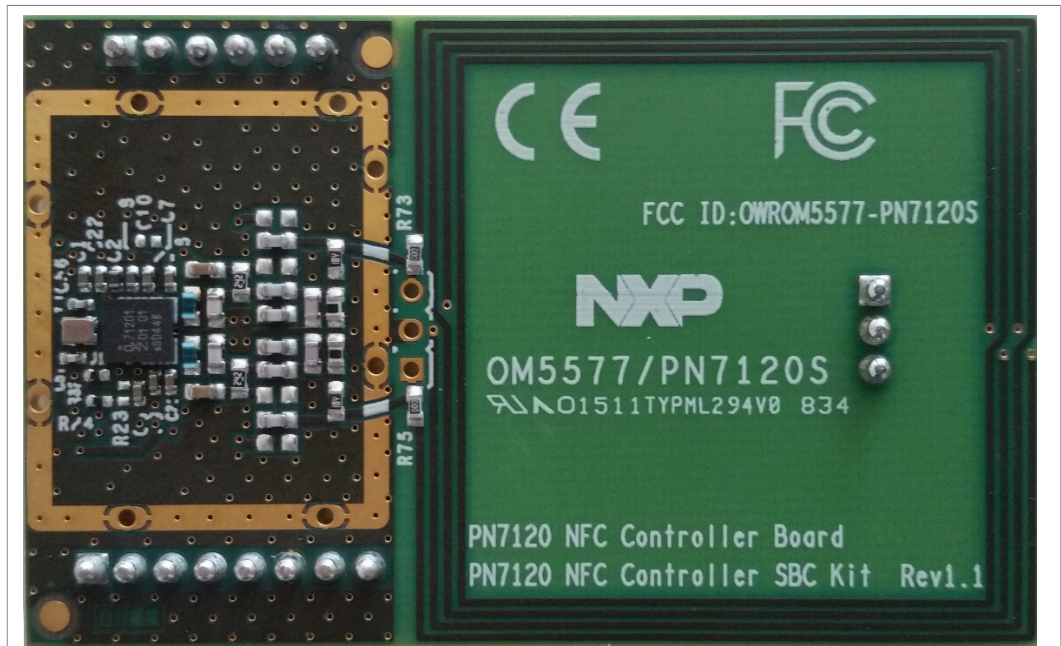
Figure 26. PN7120 NFC controller board RF antenna components
