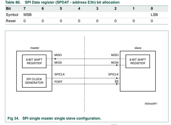
In Figure 34, SSIG (SPCTL.7) for the slave is logic 0, and  $\overline{SS}$  is used to select the slave. The SPI master can use any port pin (including P2.4/ $\overline{SS}$ ) to drive the  $\overline{SS}$  pin.
