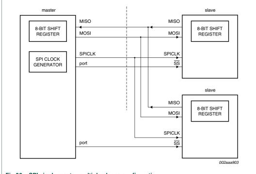
Fig 36. SPI single master multiple slaves configuration.
