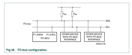
The P89LPC952/954 CPU interfaces with the I<sup>2</sup>C-bus through six Special Function Registers (SFRs): I2CON (I<sup>2</sup>C Control Register), I2DAT (I<sup>2</sup>C Data Register), I2STAT (I<sup>2</sup>C Status Register), I2ADR (I<sup>2</sup>C Slave Address Register), I2SCLH (SCL Duty Cycle Register High Byte), and I2SCLL (SCL Duty Cycle Register Low Byte).
