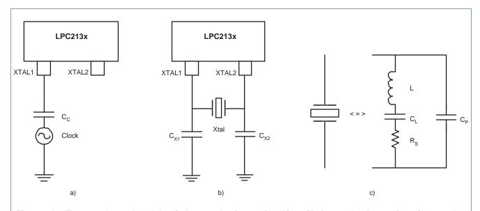
Fig 7. Oscillator modes and models: a) slave mode of operation, b) oscillation mode of operation, c) external crystal model used for  $C_{X1}/X_2$  evaluation
