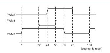
The waveforms below show a single PWM cycle and demonstrate PWM outputs under the following conditions:
