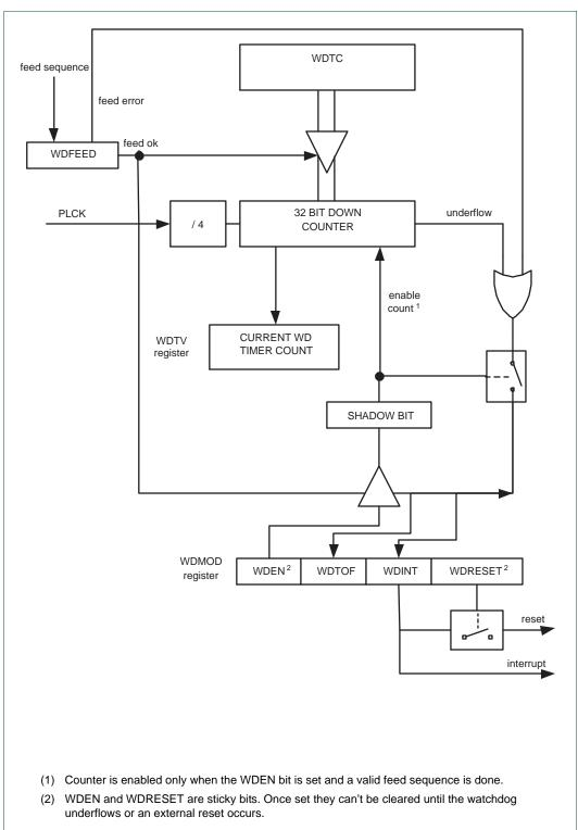
Fig 55. Watchdog block diagram
