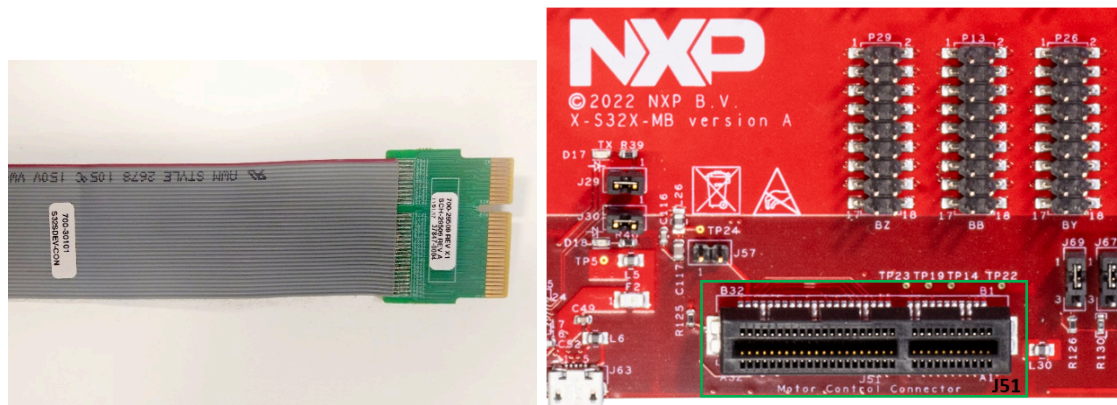
S32SDEV-CON motor control connector cable and socket
