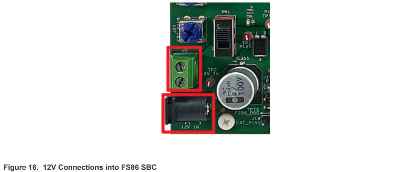
Figure 16. 12V Connections into FS86 SBC
