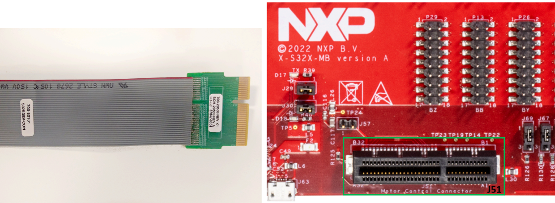
S32SDEV-CON motor control connector cable and socket
