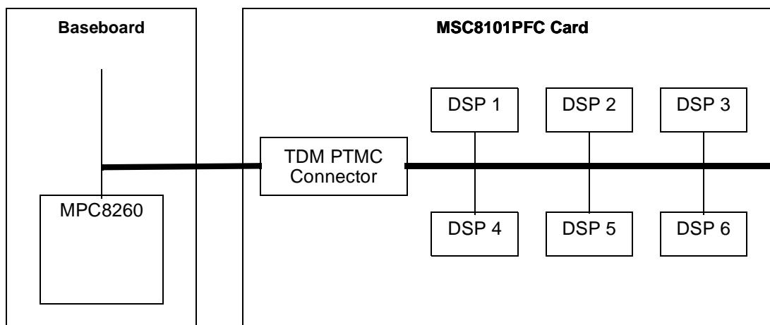
**Figure 10.** TDM Signal Path
