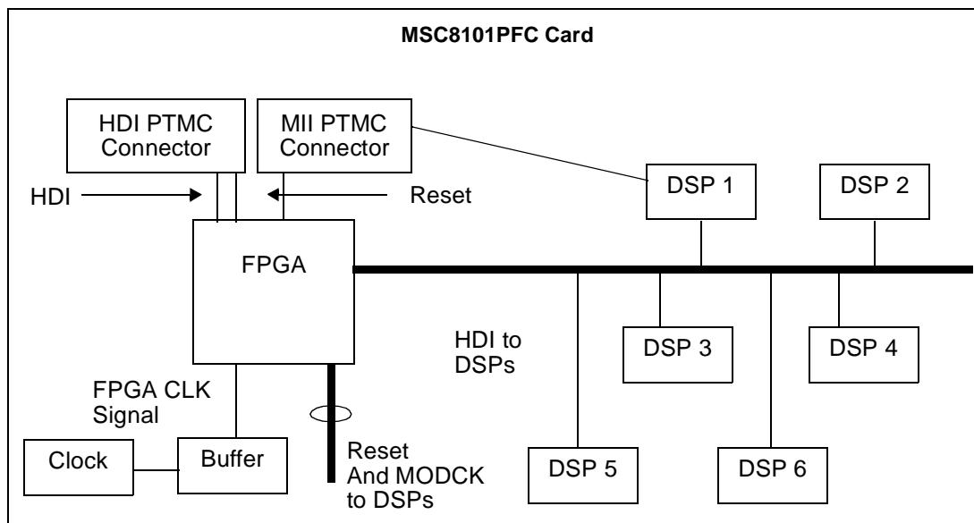
**Figure 4.** Device and Signals that Connect to FPGA
