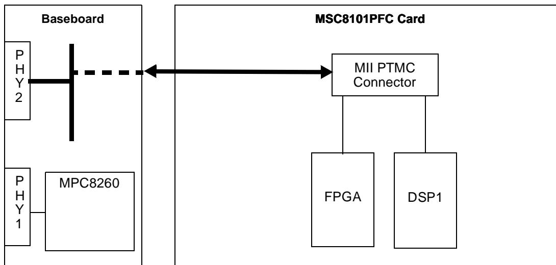
**Figure 12.** MII Path Between the MSC8101PFC Card PHY and the Baseboard
