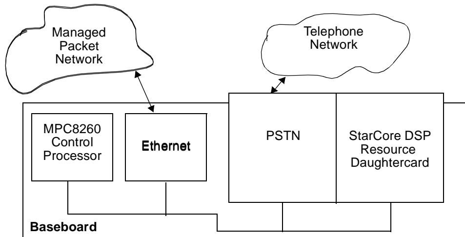
**Figure 2.** Components of the Packet Telephony Development Kit (PTK)
