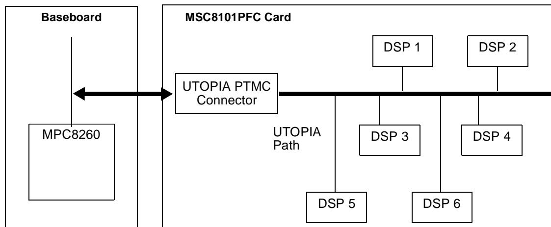
**Figure 11.** UTOPIA Path Between the Baseboard and MSC8101PFC Card**Table 12.** PTMC P4 Header
