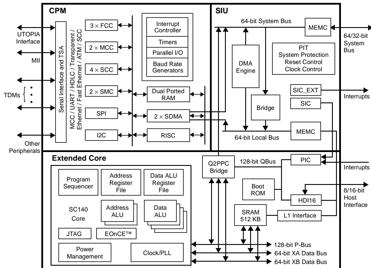
**Figure 3.** MSC8101 Block diagram
