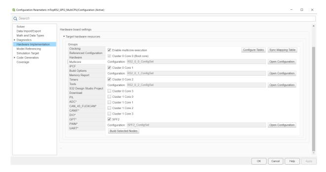
Simulink Concurrent Execution GUI can be accessed by clicking the *Configure Tasks* button. For more information about explicit partitioning in Simulink, please visit MathWorks websites Concepts in multicore programming, Setup partitions in explicit partitioning.
