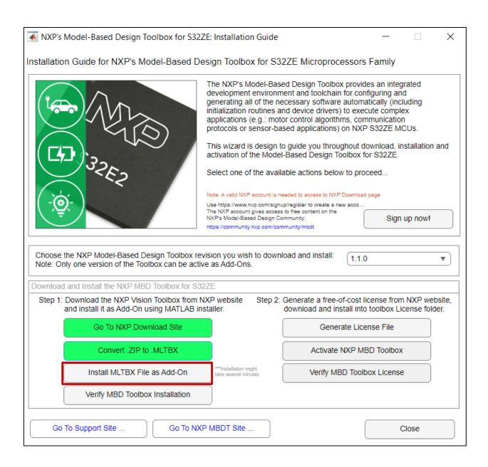
5. In the MATLAB Add-On Manager, Review the Terms and Conditions as you scroll down, and press **I Accept** Button. This action starts MBDT for S32Z/E Toolbox installation process.
