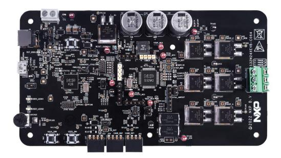
Evaluation boards must be powered via an external 12V power adapter, and an USB cable connected between the host PC and the OpenSDA USB port on the EVB. In case the OpenSDA port is not available, an external probe (P&E Micro Multilink) can be used.
