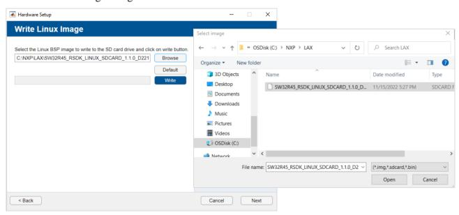
Finally, push the Write button to write the Linux image.
