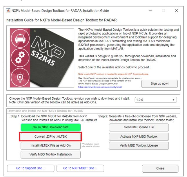
4. Go back to **NXP Toolbox Installation Guide** and select the **Install MLTBX File as Add-On** button. In the newly opened window, browse for the MLTBX file and press **Open.**
