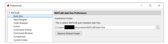
**Note:** It is recommended to install the MATLAB and NXP Toolbox in a location that does not contain special characters, empty spaces, or mapped drives.
