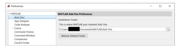
**Note:** It is recommended to install the MATLAB and NXP Toolbox in a location that does not contain special characters, empty spaces, or mapped drives.
