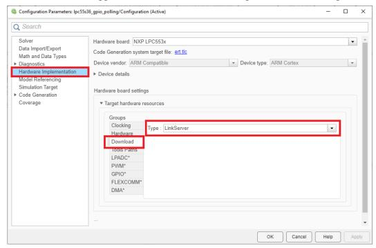
3. Press the Build Model button and wait until the code is generated, compiled, and downloaded to the evaluation board. Alternatively, you can press on the text highlighted in the model to start the process automatically.
