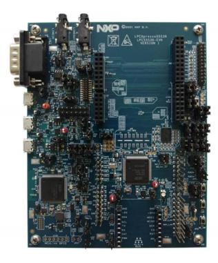
Before running any example on the **LPCXpresso55S36 Development Board**, please connect the board to the PC via a microUSB cable on the Link2 J1 USB connector.
