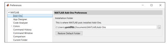
**Note:** It is recommended to install the MATLAB and NXP Toolbox into a location that does not contain special characters, empty spaces, or mapped drives.
