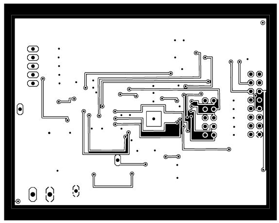
Figure 3. Bottom Copper Layer (As Seen Thru Board Looking From The Top)
