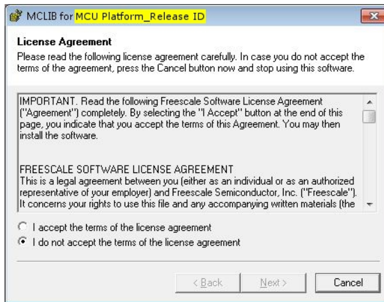
Figure 2-4. MCLib installation - step 1. Highlighted "releaseID" identifies the actual release number, which is MCLIB for MPXR40xx
