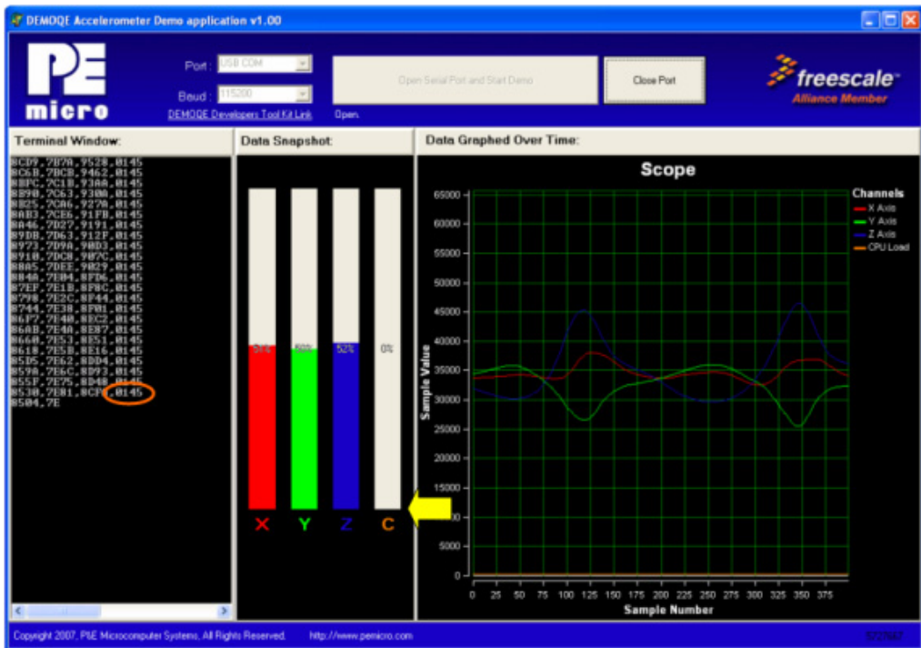
Figure 3-10: Accelerometer Demo running on 32-bit ColdFire V1 QE128 in data averaging mode. Yellow arrow highlights the bus cycles required to average the last 16 readings of the 3 axes. Value shown in orange circle is the number of bus cycles in hex.
