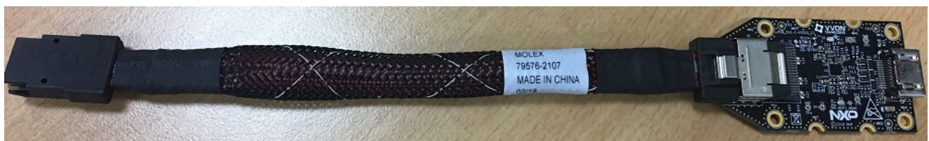
Figure 11. i.MX mini SAS cable with DSI-to-HDMI adapter
