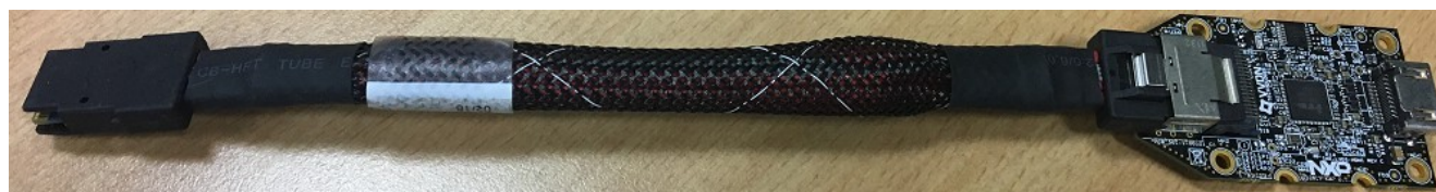
Figure 24. i.MX mini SAS cable with LVDS-to-HDMI adapter
