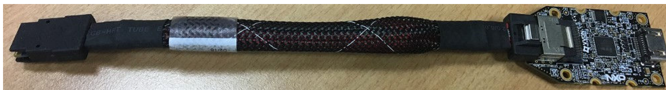
Figure 12. i.MX mini SAS cable with LVDS-to-HDMI adapter
