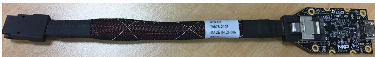
Figure 23. i.MX mini SAS cable with DSI-to-HDMI adapter
