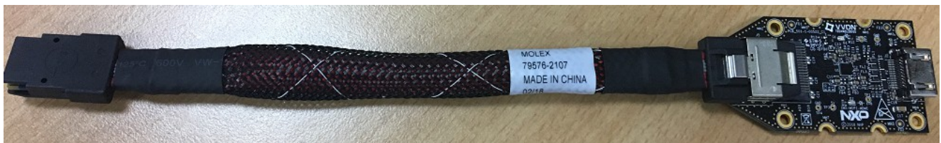
Figure 28. i.MX mini SAS cable with DSI-to-HDMI adapter
