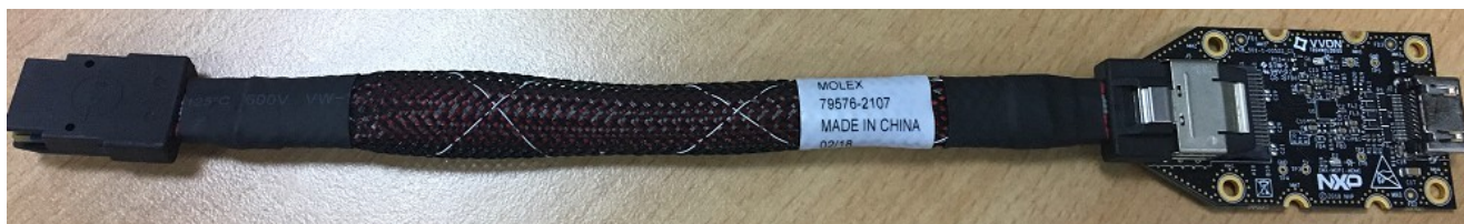
Figure 7. i.MX mini SAS cable with DSI-to-HDMI adapter
