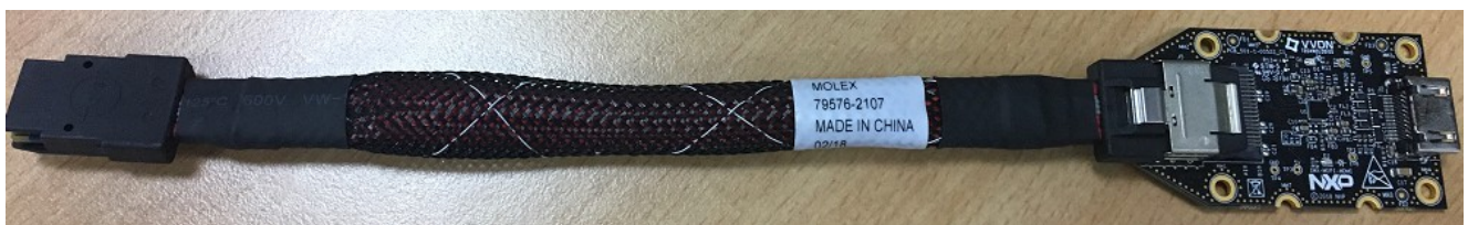
Figure 11. i.MX mini SAS cable with DSI-to-HDMI adapter
