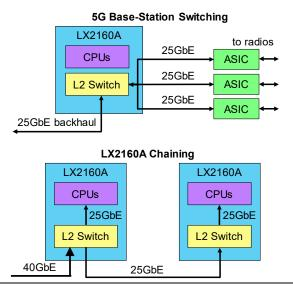
**Figure 2. Two common examples of LX2160A switching.** In the first case, the processor distributes incoming packets to multiple ASICs in a base station. In the second case, one processor separates the incoming traffic and distributes some of it to a chained processor.
