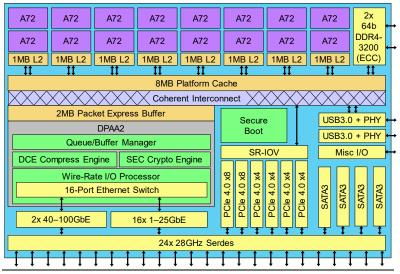
**Figure 1. Block diagram of NXP QorIQ LX2160A.** In addition to 16 CPUs, major features include 100G Ethernet, a 16-port Ethernet switch, large ECC-protected caches and buffers, PCI Express Gen4, and faster accelerators for cryptography and compression.
