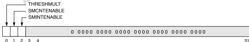
Figure 11-3. Monitor Mode Control Register 2 (MMCR2)
