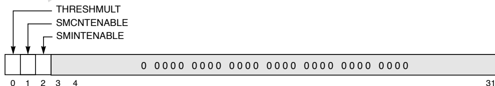
Figure 2-7. Monitor Mode Control Register 2 (MMCR2)
