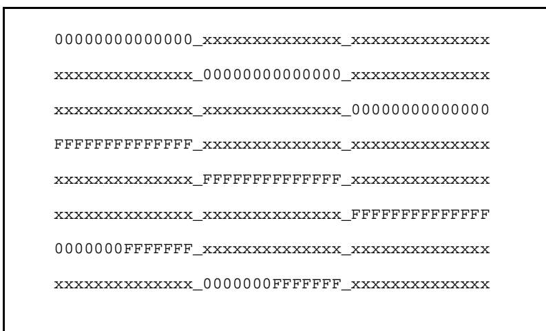
Figure 14-29. Known Weak SCC Key Patterns
