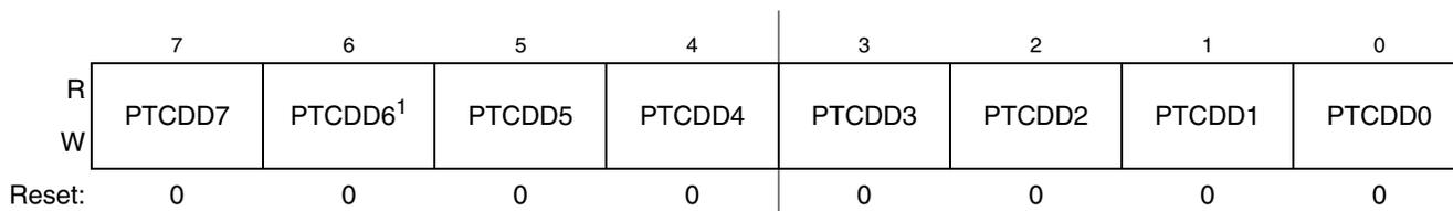
Figure 6-13. Port C Data Direction Register (PTCDD)
