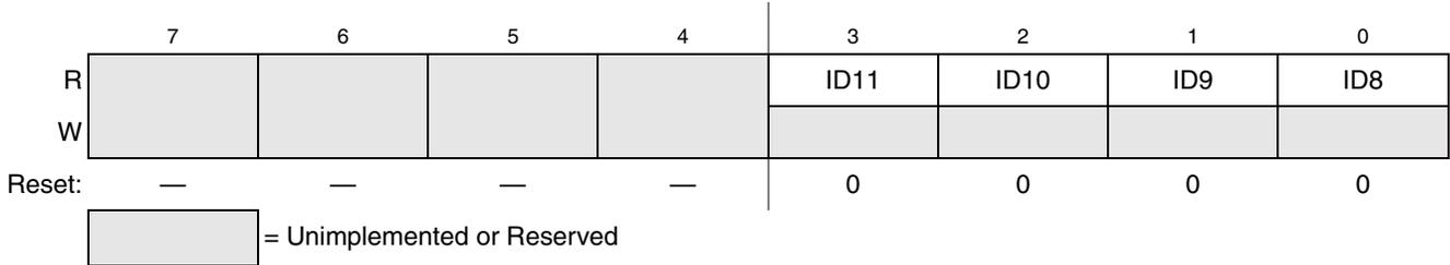
Figure 5-7. System Device Identification Register — High (SDIDH)
