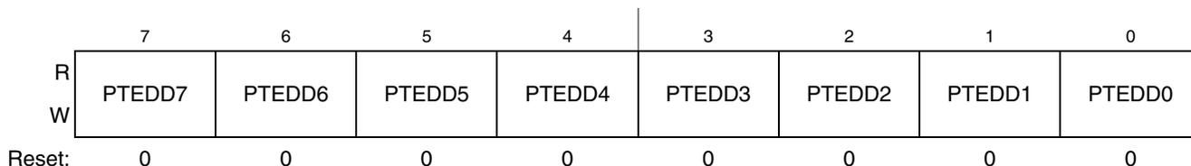
Figure 6-23. Port E Data Direction Register (PTEDD)
