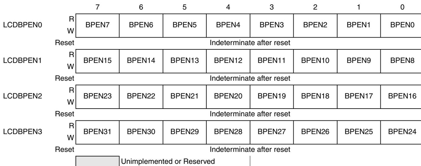
**Figure 13-10. Backplane Enable Registers 0–3 (LCDBPEN0–LCDBPEN3)**
