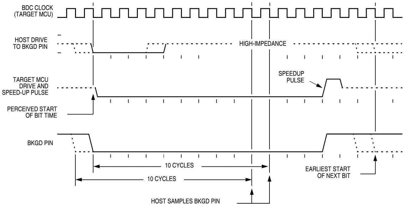
Figure 18-4. BDM Target-to-Host Serial Bit Timing (Logic 0)
