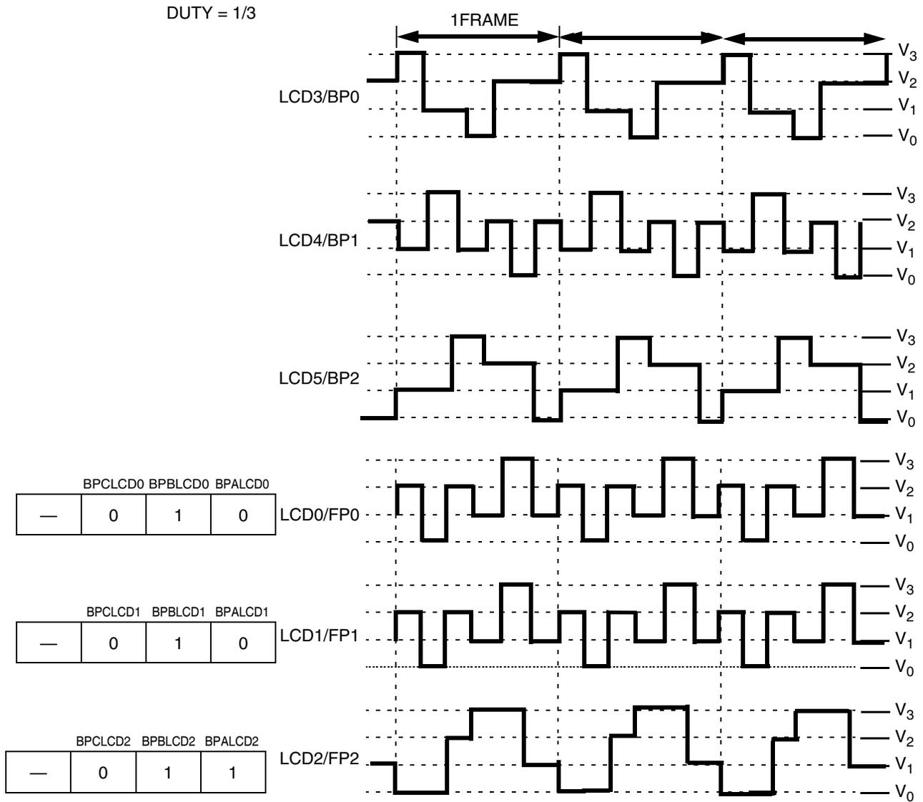
Figure 13-19. LCD Waveforms
