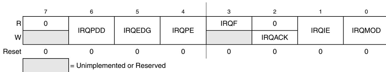
**Figure 5-2. Interrupt Request Status and Control Register (IRQSC)**
