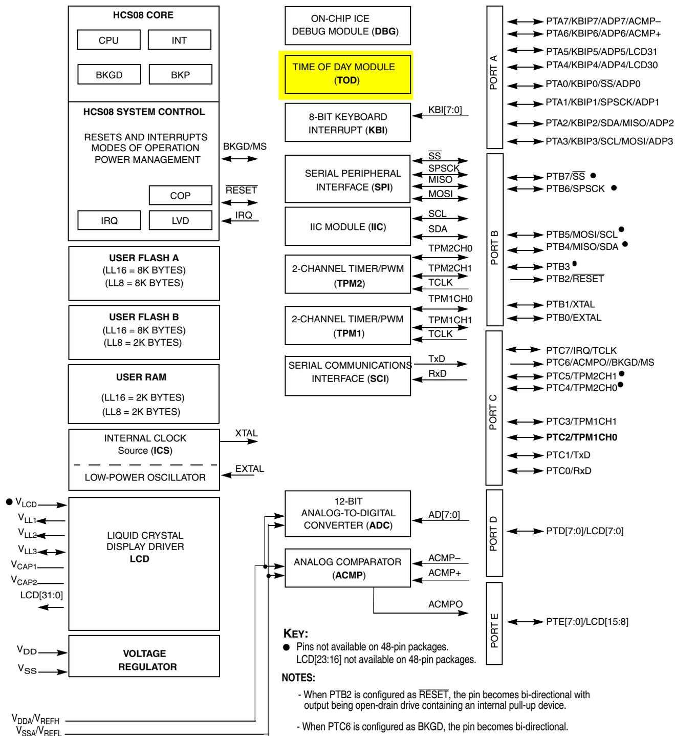
Figure 17-1. MC9S08LL16 Block Diagram Highlighting TOD Block
