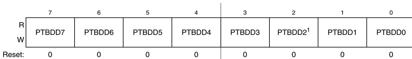
Figure 6-8. Port B Data Direction Register (PTBDD)
