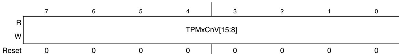
**Figure 16-13. TPM Channel Value Register High (TPMxCnVH)**
