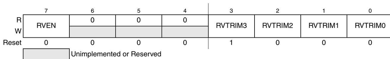
**Figure 13-6. LCD Regulated Voltage Control Register (LCDRVC)**
