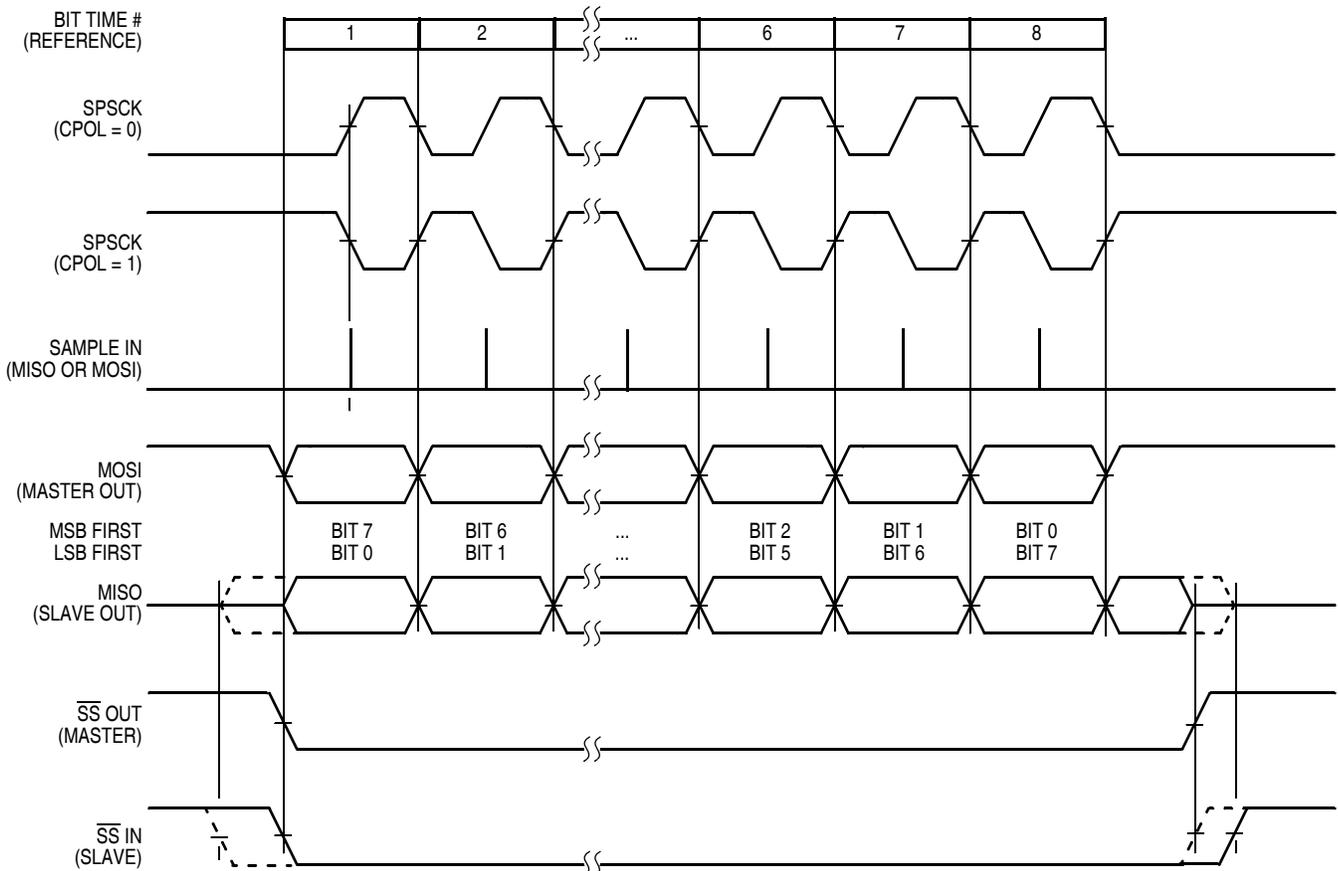
Figure 15-11. SPI Clock Formats (CPHA = 0)
