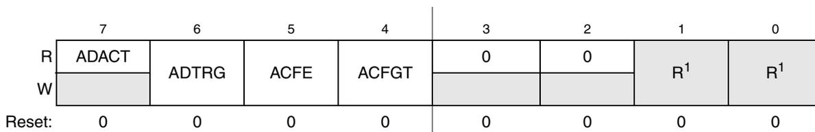
**Figure 10-4. Status and Control Register 2 (ADCSC2)**
