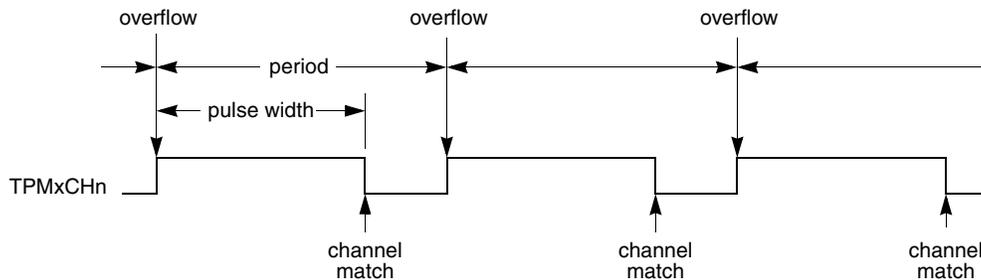
Figure 16-15. EPWM period and pulse width (ELSnA=0)
