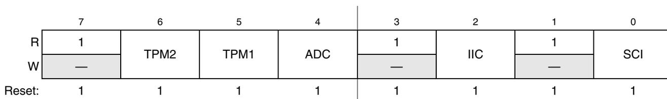
Figure 5-12. System Clock Gating Control 1 Register (SCGC1)
