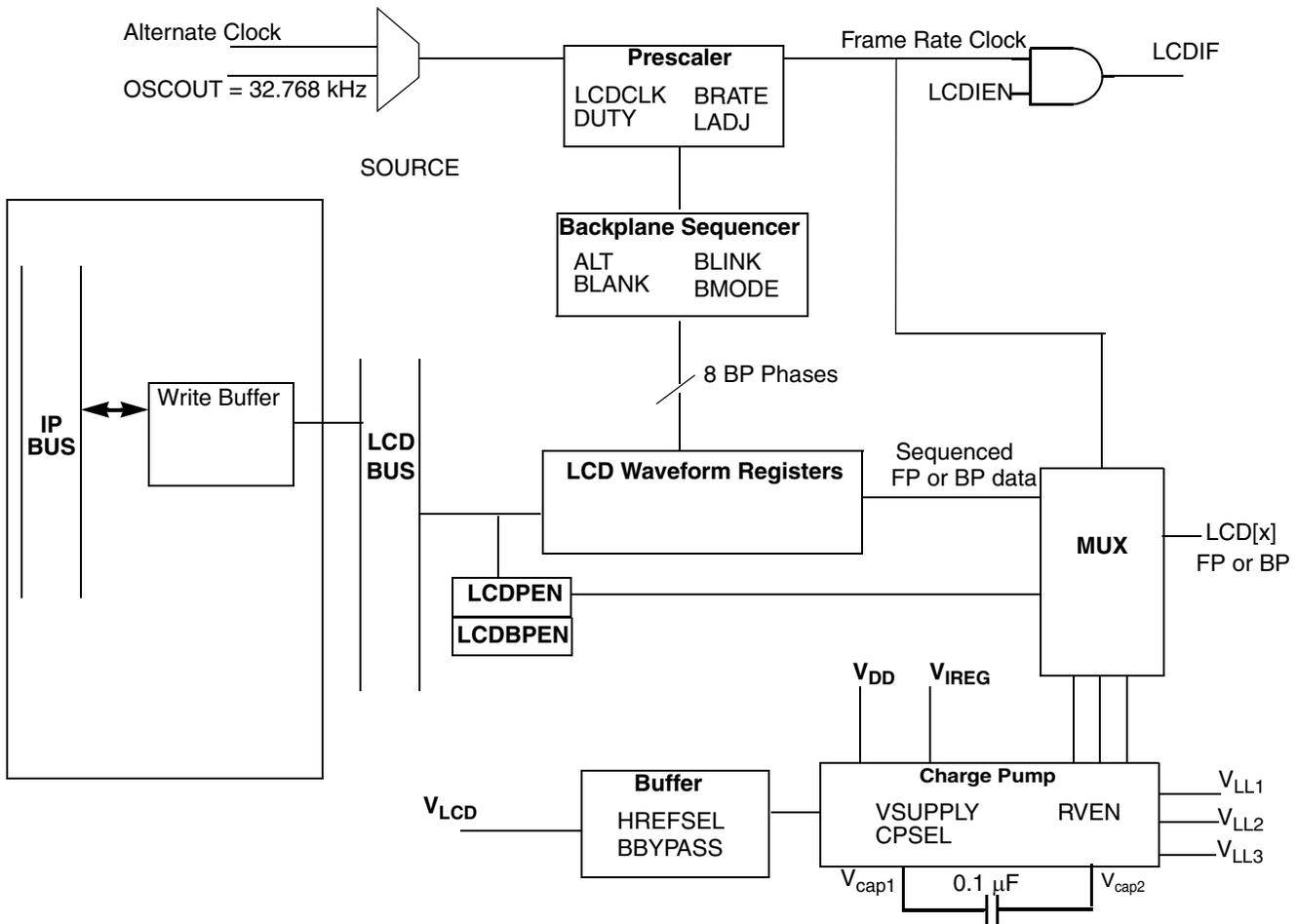
Figure 13-2. LCD Driver Block Diagram
