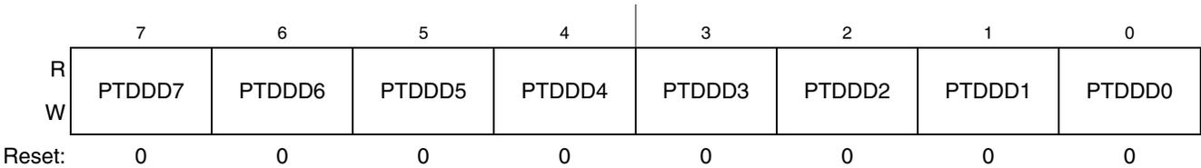
Figure 6-18. Port D Data Direction Register (PTDDD)
