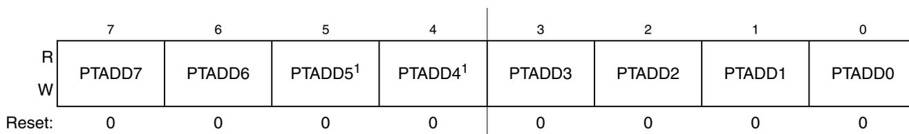
**Figure 6-3. Port A Data Direction Register (PTADD)**
