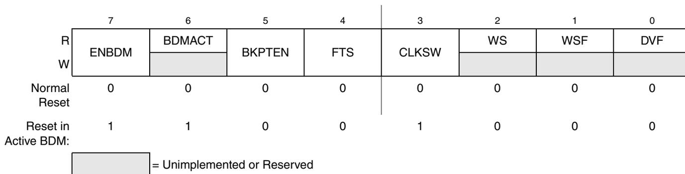
**Figure 18-5. BDC Status and Control Register (BDCSCR)**
