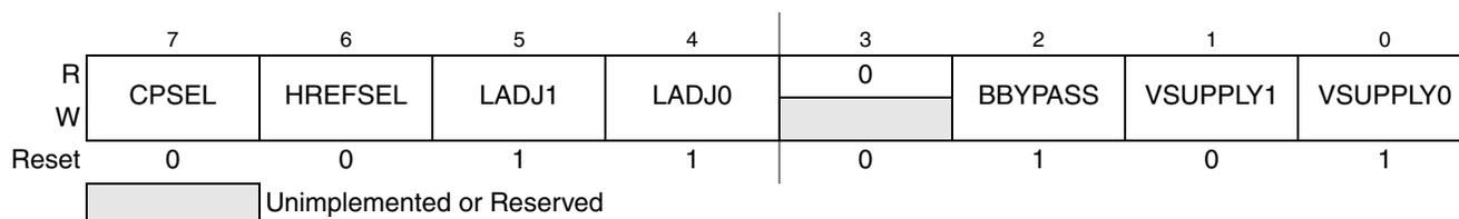
Figure 13-5. LCD Voltage Supply Register (LCDSUPPLY)
