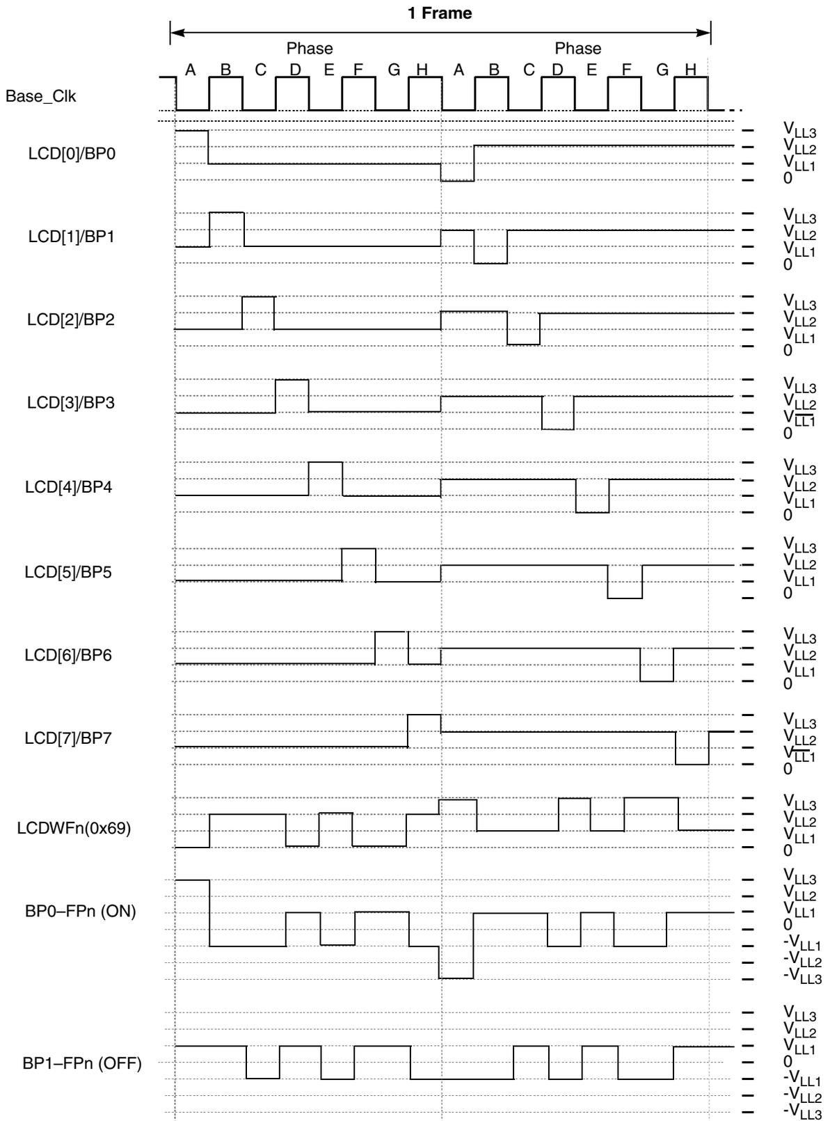
Figure 13-15. 1/8 Duty and 1/3 Bias (Low-power Waveform)
