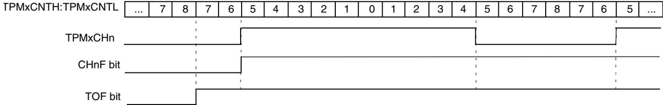
**Figure 16-5. High-true pulse of a center-aligned PWM**
