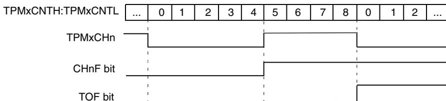
**Figure 16-4. Low-true pulse of an edge-aligned PWM**
