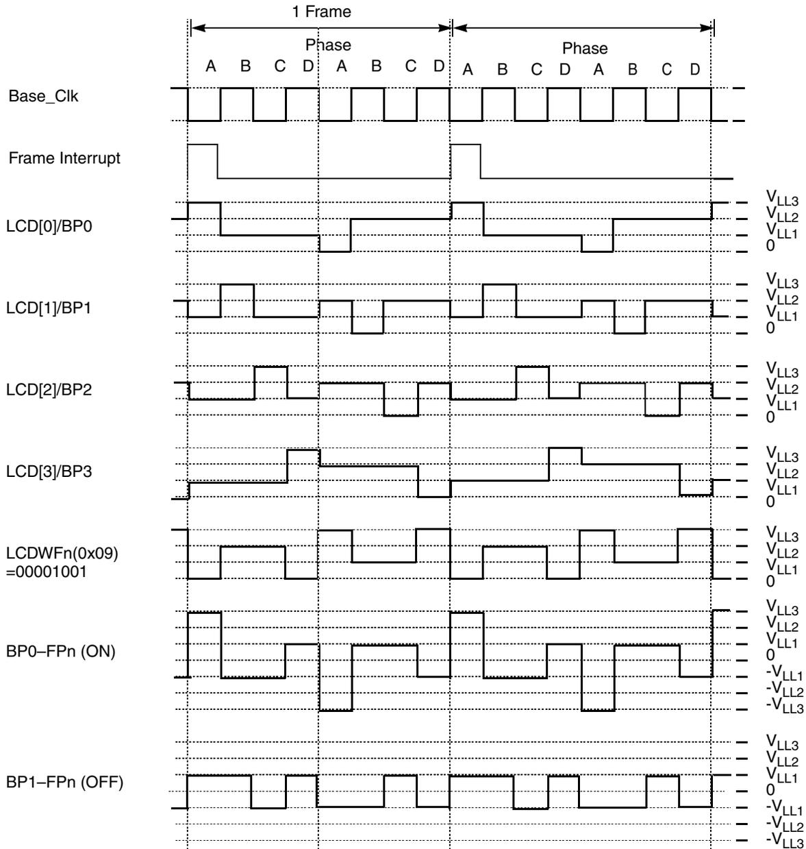
Figure 13-14. 1/4 Duty and 1/3 Bias (Low-Power Waveform)
