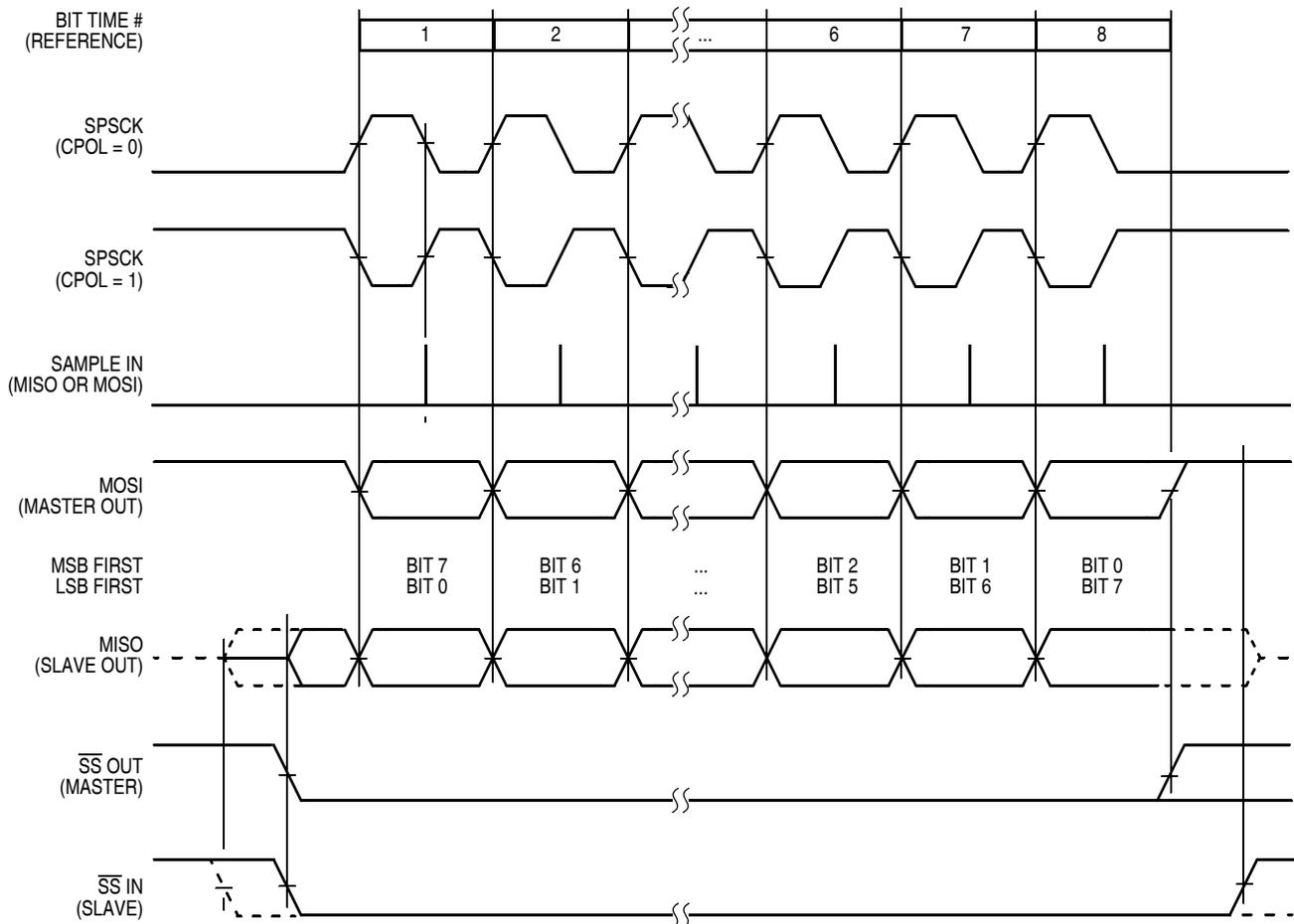
Figure 15-10. SPI Clock Formats (CPHA = 1)
