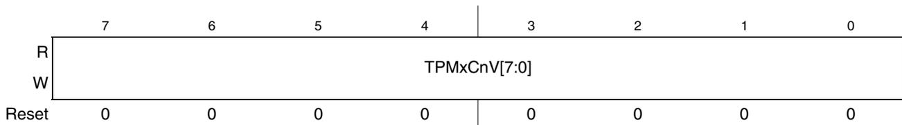
**Figure 16-14. TPM Channel Value Register Low (TPMxCnVL)**
