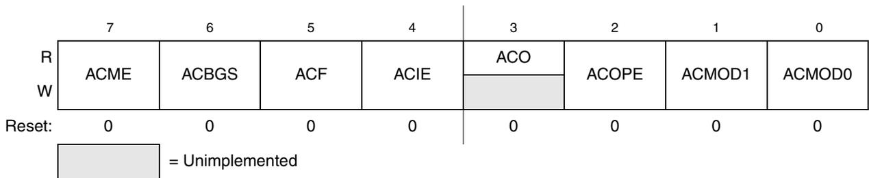
Figure 9-3. ACMP Status and Control Register (ACMPSC)
