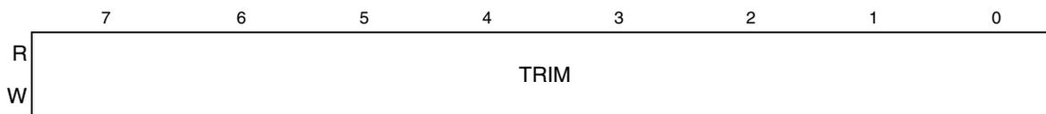
Reset: Note: TRIM is loaded during reset from a factory programmed location when not in BDM mode. If in a BDM mode, a default value of 0x80 is loaded.
