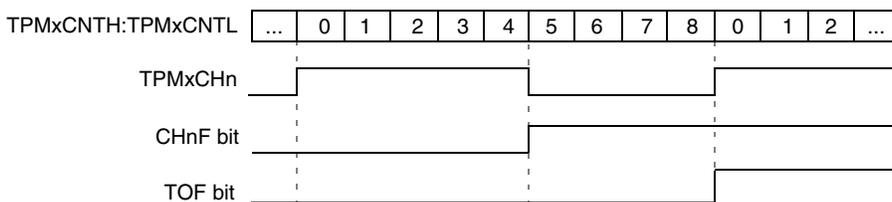
**Figure 16-3. High-true pulse of an edge-aligned PWM**
