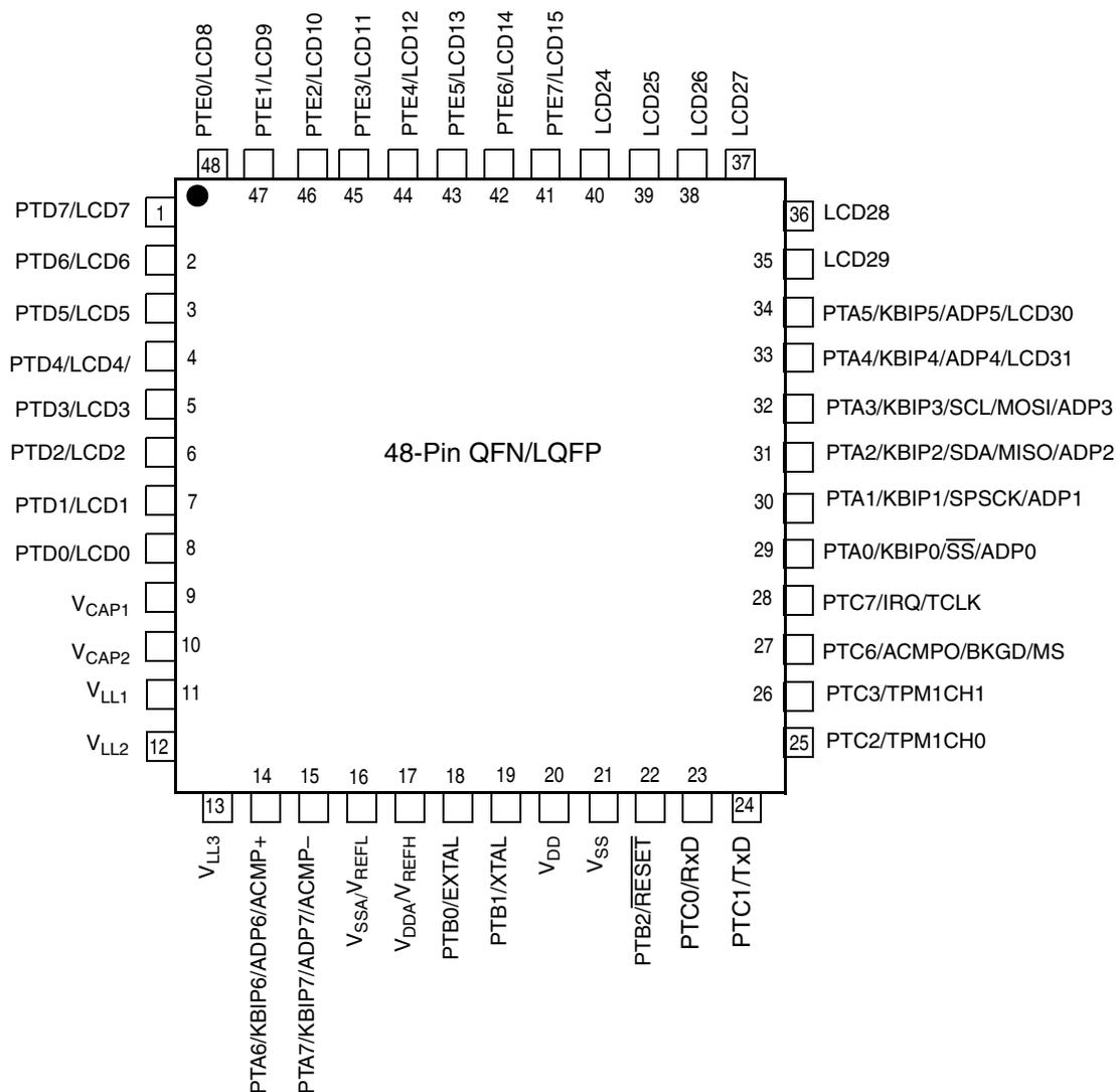
Note: V<sub>REFH</sub>/V<sub>REFL</sub> are internally connected to V<sub>DDA</sub>/V<sub>SSA</sub>
