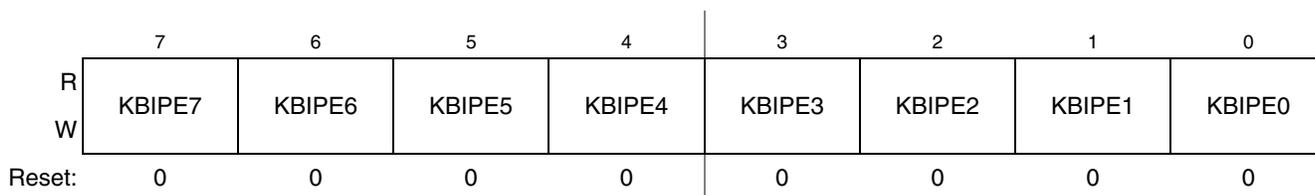
Figure 7-4. KBI Interrupt Pin Select Register (KBIPE)
