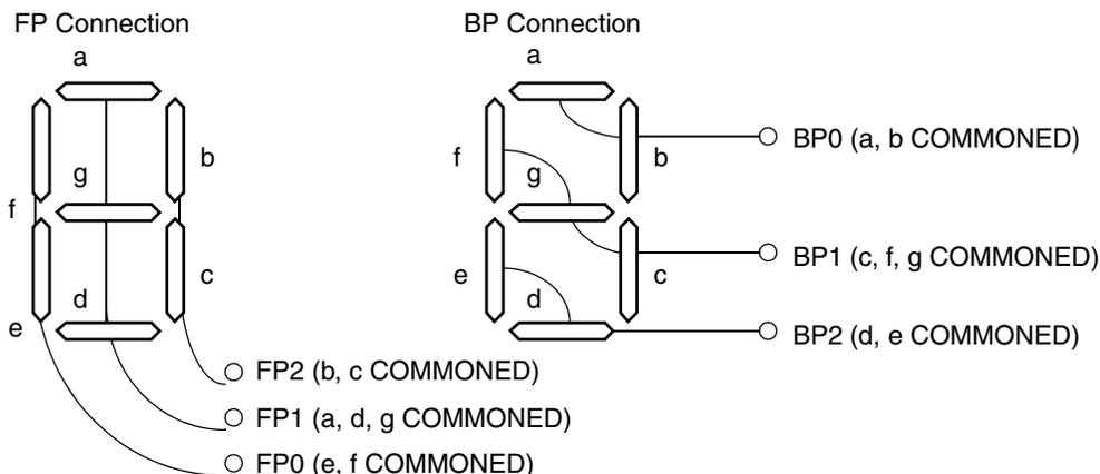
The above segment assignments are provided by the specification for the LCD glass for this example. For this LCD Module any of the LCD pins can be configured to be Frontplane 0-2 or Backplane 0-2. For this example we will set LCD[0] as FP0, LCD[1] as FP1, and LCD[2] as FP2. For this example we will set LCD[3] as BP0, LCD[4] as BP1 and LCD[5] as BP2.
