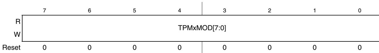
Figure 16-11. TPM Counter Modulo Register Low (TPMxMODL)
