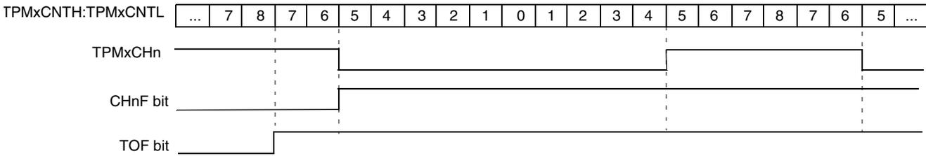
**Figure 16-6. Low-true pulse of a center-aligned PWM**
