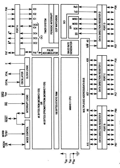
\*PA6 and PA4 not bonded in 40 pin DIP
