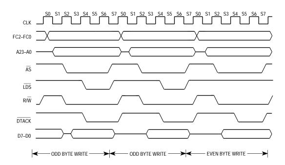
Figure 4-4. Write-Cycle Timing Diagram
