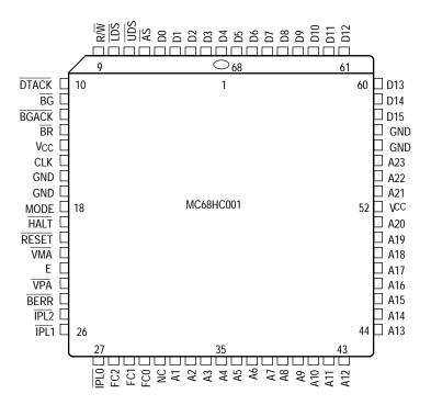
Figure 11-3. 68-Lead Quad Pack (2 of 2)
