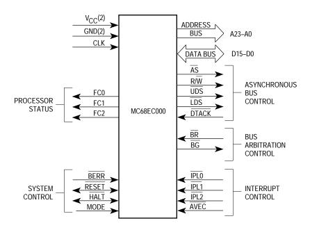
Figure 3-3. Input and Output Signals (MC68EC000)
