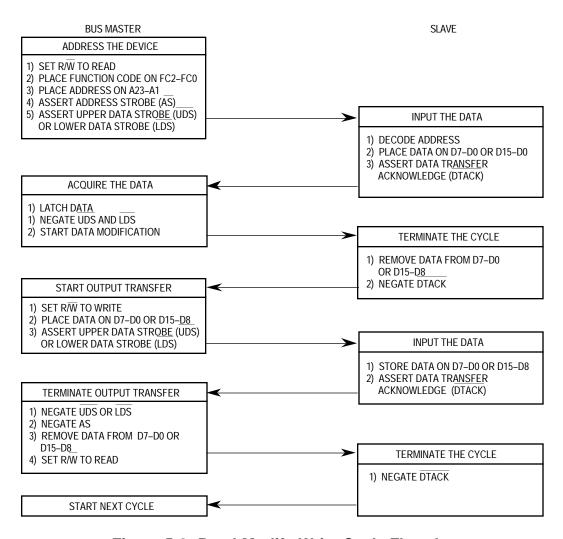
Figure 5-8. Read-Modify-Write Cycle Flowchart
