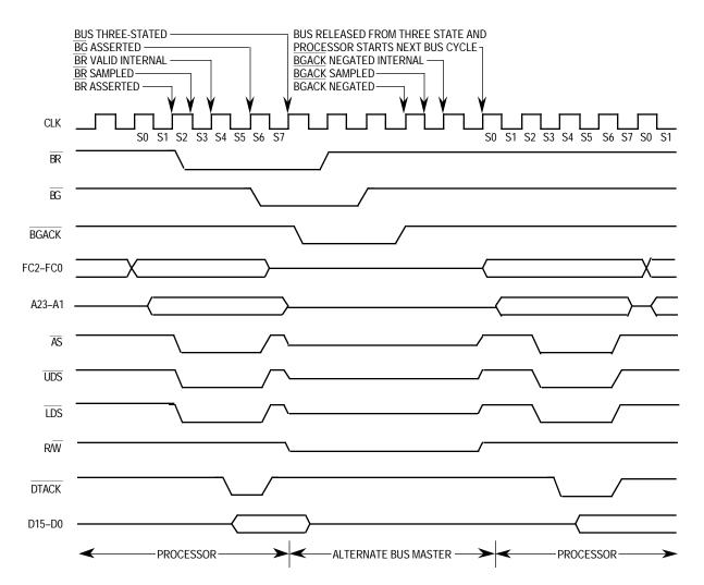
Figure 5-19. 3-Wire Bus Arbitration Timing Diagram—Processor Active
