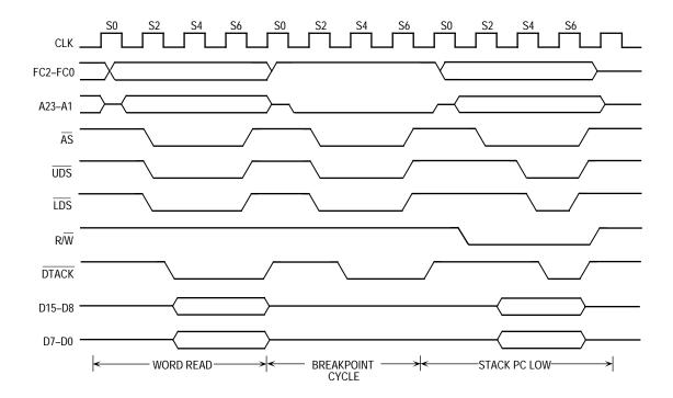
Figure 5-12. Breakpoint Acknowledge Cycle Timing Diagram
