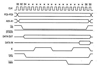
Figure B-5. M6800 Peripheral Timing—Worst Case
