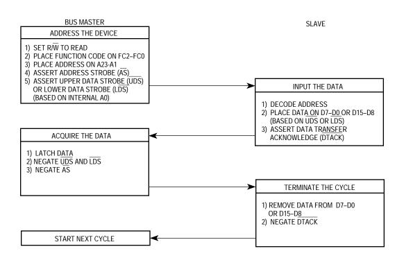
Figure 5-2. Byte Read-Cycle Flowchart
