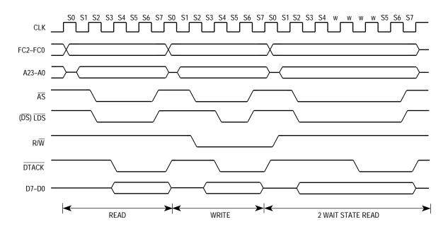
Figure 4-2. Read and Write-Cycle Timing Diagram
