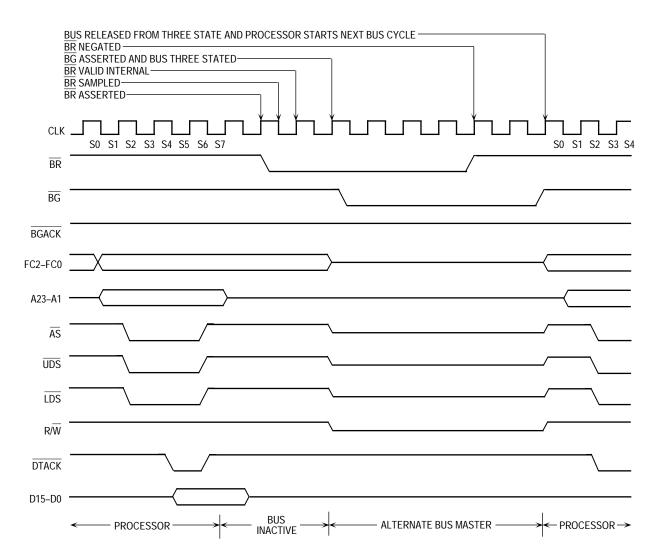
Figure 5-23. 2-Wire Bus Arbitration Timing Diagram—Bus Inactive
