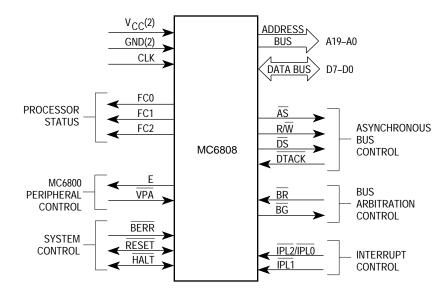
Figure 3-4. Input and Output Signals (MC68008, 48-Pin Version)
