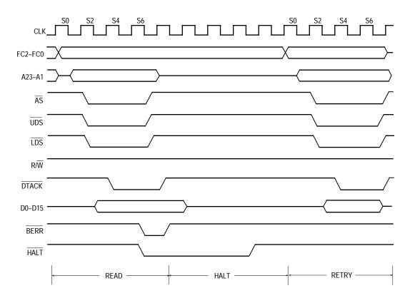
Figure 5-29. Halt Operation Timing Diagram
