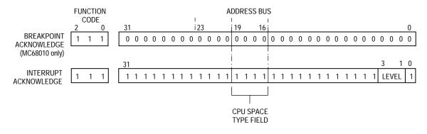
Figure 5-10. CPU Space Address Encoding
