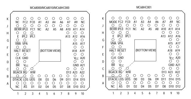
Figure 11-2. 68-Lead Pin Grid Array
