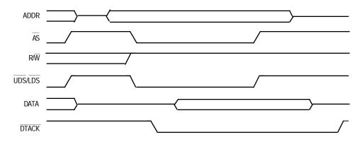
Figure 5-31. Fully Asynchronous Read Cycle
