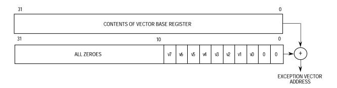
Figure 6-4. Exception Vector Address Calculation (MC68010)
