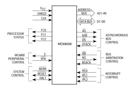
Figure 3-5. Input and Output Signals (MC68008, 52-Pin Version)
