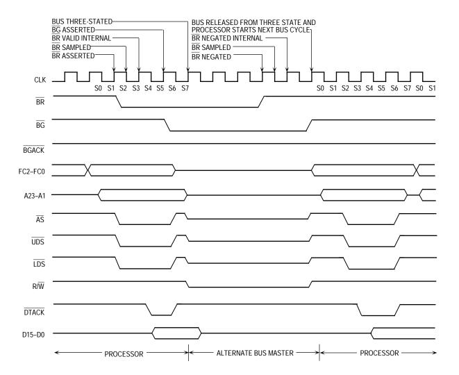
Figure 5-22. 2-Wire Bus Arbitration Timing Diagram—Processor Active
