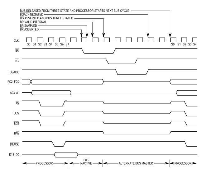
Figure 5-20. 3-Wire Bus Arbitration Timing Diagram—Bus Inactive
