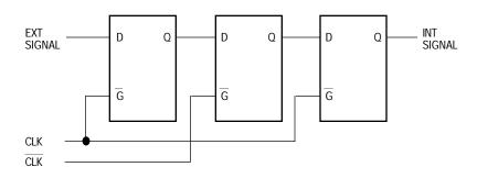
Figure 5-37. Input Synchronizers
