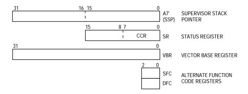
Figure 2-3. Supervisor Programmer's Model Supplement (MC68010)
