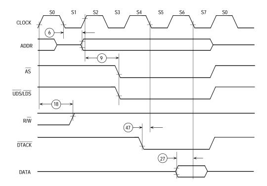
Figure 5-35. Synchronous Read Cycle
