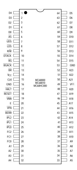
Figure 11-1. 64-Pin Dual In Line
