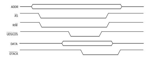
Figure 5-32. Fully Asynchronous Write Cycle
