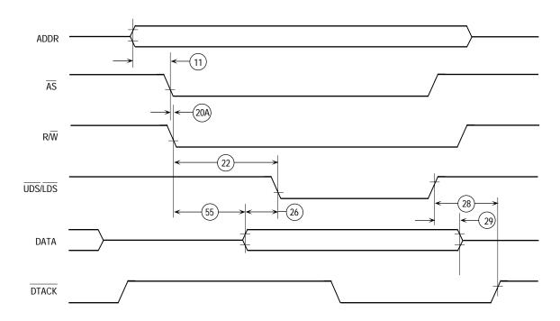
Figure 5-34. Pseudo-Asynchronous Write Cycle
