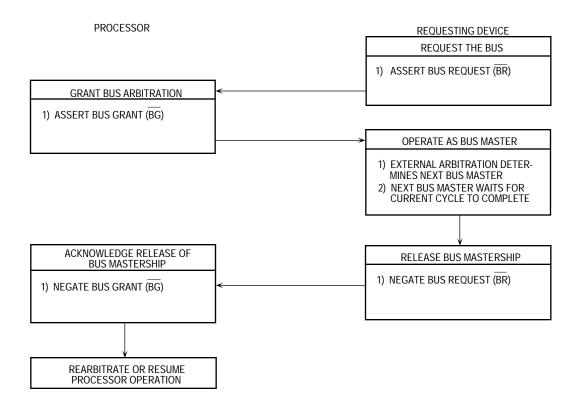
Figure 5-14. 2-Wire Bus Arbitration Cycle Flowchart
