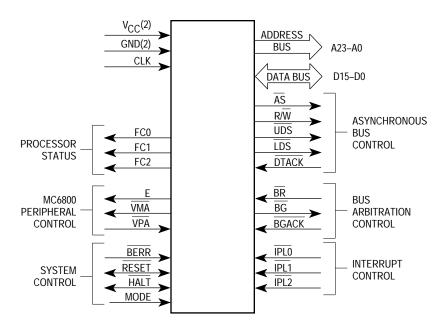
Figure 3-2. Input and Output Signals (MC68HC001)
