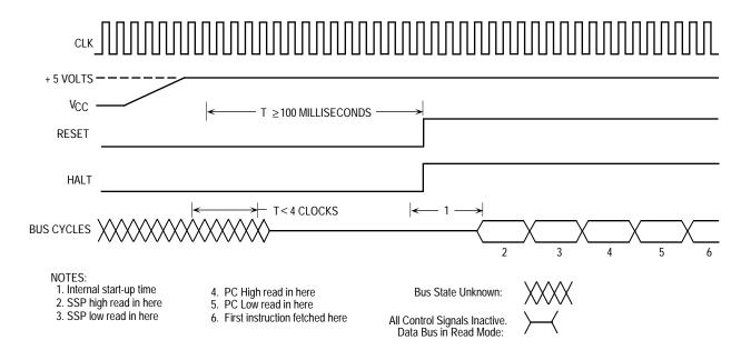
Figure 5-30. Reset Operation Timing Diagram
