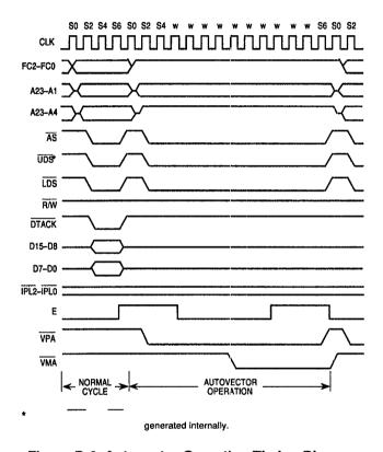
Figure B-6. Autovector Operation Timing Diagram
