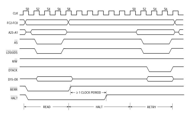
Figure 5-27. Retry Bus Cycle Timing Diagram
