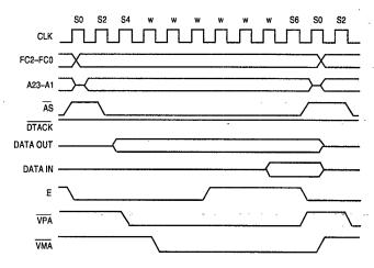
Figure B-4 M6800 Peripheral Timing—Best Case
