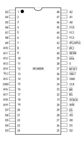
Figure 11-5. 48-Pin Dual In Line
