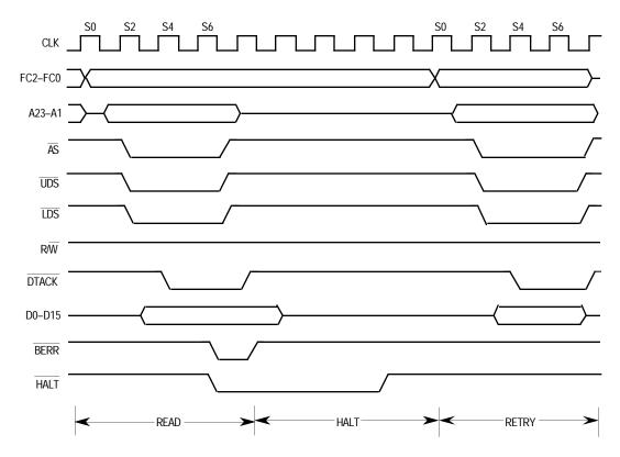
Figure 5-28. Delayed Retry Bus Cycle Timing Diagram
