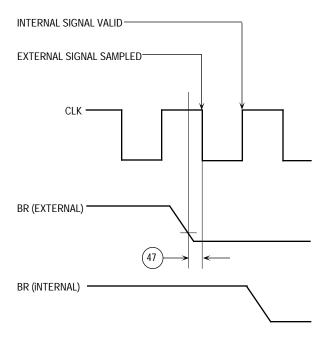
Figure 5-17. External Asynchronous Signal Synchronization
