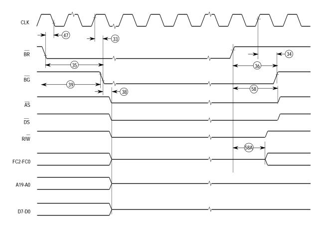
NOTES: Waveform measurements for all inputs and outputs are specified at: logic high 2.0 V, logic low = 0.8 V.
