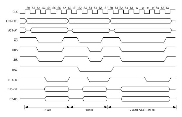
Figure 5-3. Read and Write-Cycle Timing Diagram
