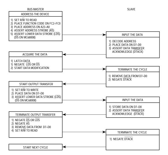
Figure 4-5. Read-Modify-Write Cycle Flowchart
