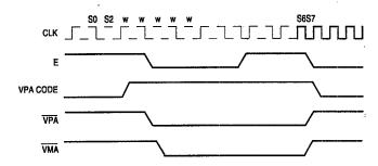
Figure B-3 External VMA Timing
