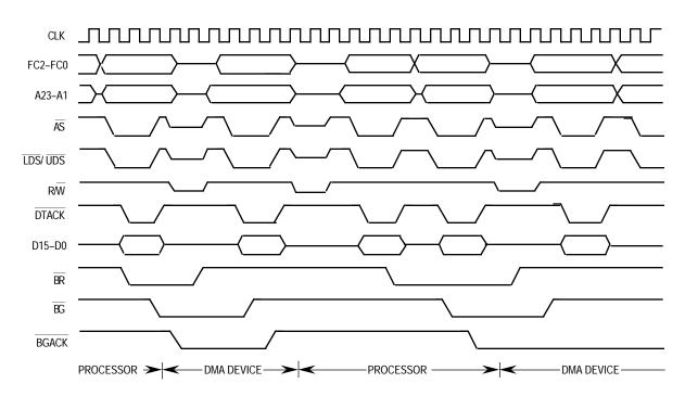
Figure 5-15. 3-Wire Bus Arbitration Timing Diagram (Not Applicable to 48-Pin MC68008 or MC68EC000)
