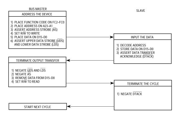
Figure 5-5. Word Write-Cycle Flowchart
