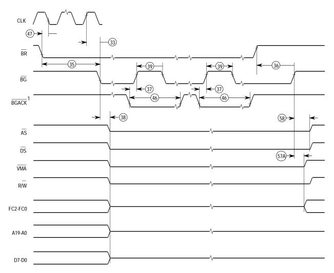
NOTES: Waveform measurements for all inputs and outputs are specified at: logic high 2.0 V, logic low = 0.8 V. 1. MC68008 52-Pin Version only.
