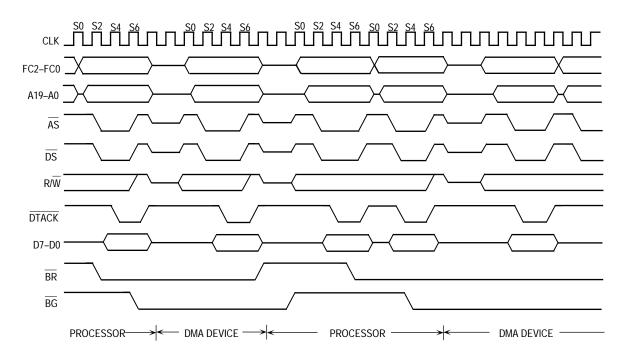
Figure 5-16. 2-Wire Bus Arbitration Timing Diagram
