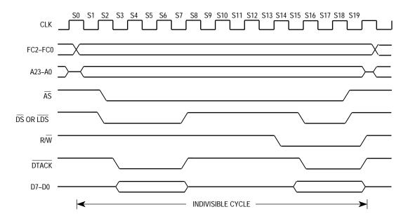
Figure 4-6. Read-Modify-Write Cycle Timing Diagram
