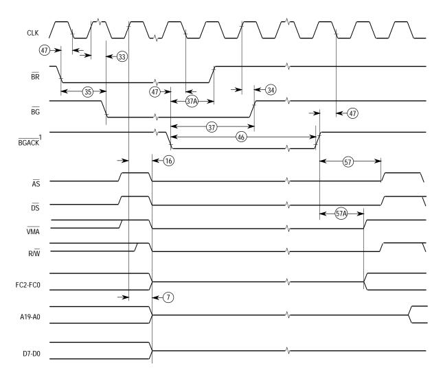
NOTE: Waveform measurements for all inputs and outputs are specified at: logic high 2.0 V, logic low = 0.8 V. 1 MC68008 52-Pin Version Only.
