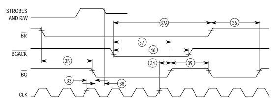
NOTE: Setup time to the clock (#47) for the asynchronous inputs  $\overline{\text{BERR}}$ ,  $\overline{\text{BGACK}}$ ,  $\overline{\text{BR}}$ ,  $\overline{\text{DTACK}}$ ,  $\overline{\text{IPL2}}$ - $\overline{\text{IPL0}}$ , and  $\overline{\text{VPA}}$  guarantees their recognition at the next falling edge of the clock.
