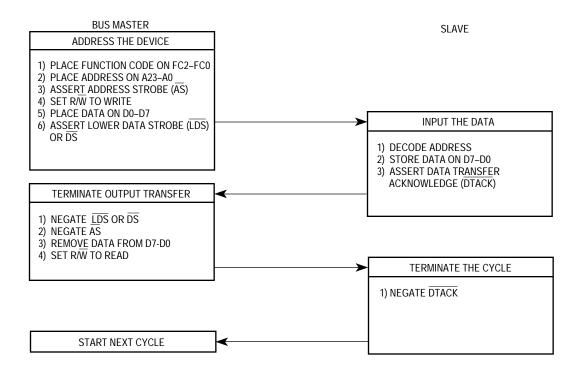
Figure 4-3. Byte Write-Cycle Flowchart
