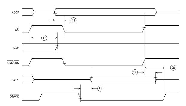
Figure 5-33. Pseudo-Asynchronous Read Cycle
