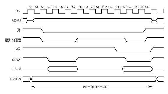
Figure 5-9. Read-Modify-Write Cycle Timing Diagram
