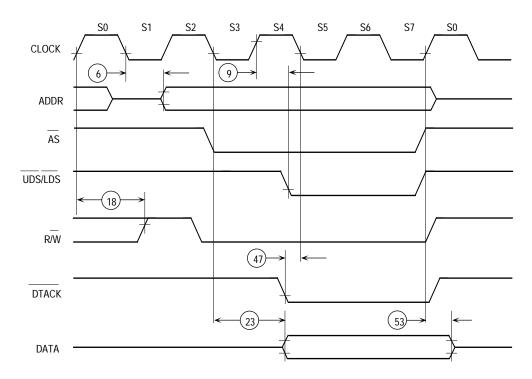
Figure 5-36. Synchronous Write Cycle
