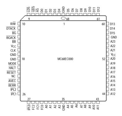
Figure 11-3. 68-Lead Quad Pack (1 of 2)
