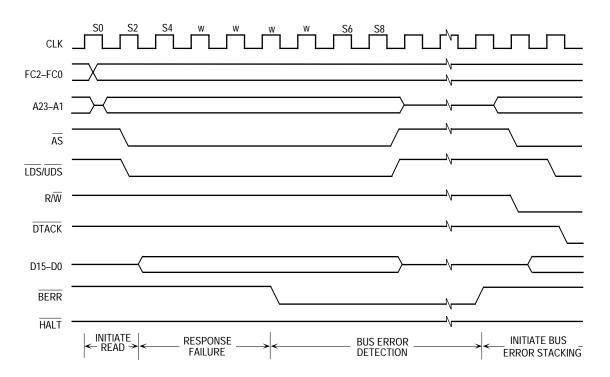
Figure 5-25. Bus Error Timing Diagram
