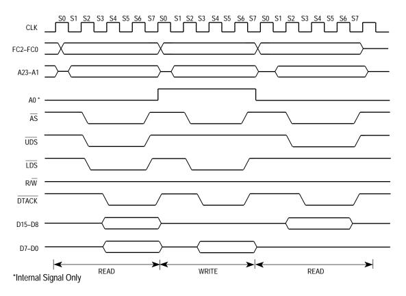
Figure 5-4. Word and Byte Read-Cycle Timing Diagram
