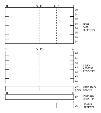
Figure 2-1. User Programmer's Model (MC68000/MC68HC000/MC68008/MC68010)
