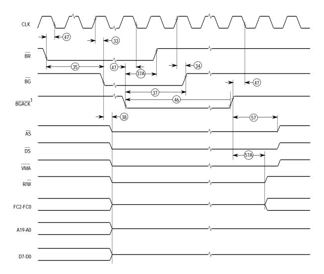
NOTES: Waveform measurements for all inputs and outputs are specified at: logic high 2.0 V, logic low = 0.8 V. 1. MC68008 52-Pin Version only.
