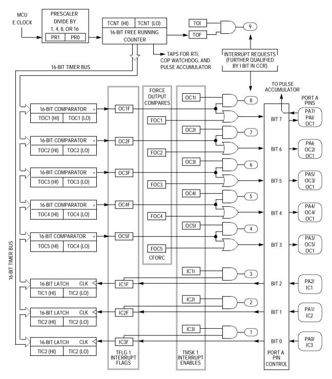
Figure 10-1. Main Timer System Block Diagram
