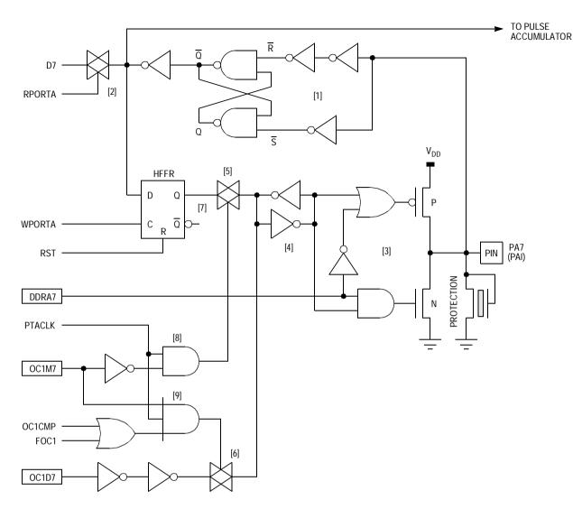
Figure 7-6. PA7 (OC1 and PAI) Pin Logic
