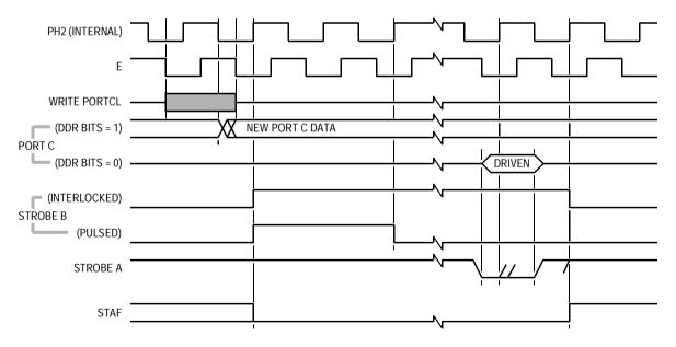
Figure 7-27. Idealized Timing for Full-Output Handshake
