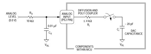
$R_X$  and  $C_X$  are the external components,  $C_i$  is the internal DAC capacitance, and  $R_i$  is the internal series resistance (includes N-channel couplers and polysilicon interconnections). From Figure 12-7,  $C_i$  is 20 pF and  $R_i$  is  $\leq 4~k\Omega$ . The switch represents an analog switch closed only during the sample time. For the chosen E-clock rate, the sample time is 6  $\mu$ s, and the period from one sample to the next sample of the same channel is 64  $\mu$ s.
