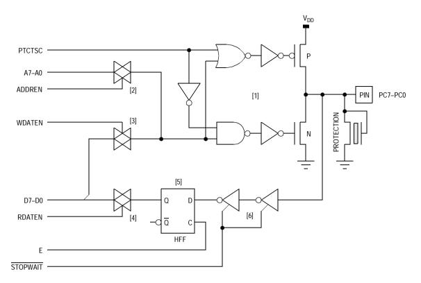
Figure 7-11. Port C Expanded Mode Pin Logic
