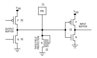
Figure 2-17. Internal Circuitry — Digital I/O Pin
