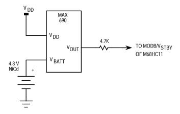
Figure 2-8. RAM Standby MODB/V<sub>STBY</sub> Connections
