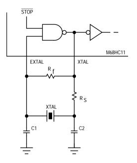
Figure 2-10. Low-Frequency Crystal Connections
