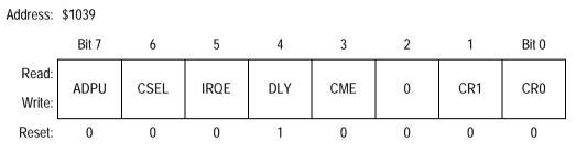
Figure 3-5. System Configuration Option Register (OPTION)
