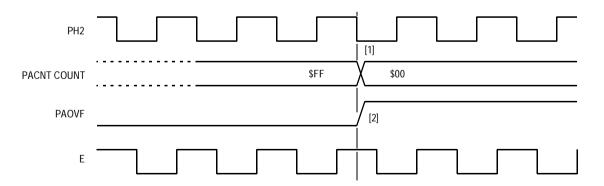
Figure 11-12. Timing Details for Pulse Accumulator Counter Overflow
