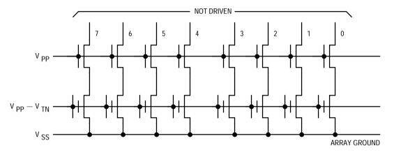
Figure 4-5. Erasing an EEPROM Byte
