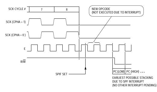
Figure 8-8. Transfer Ending for an SPI Master
