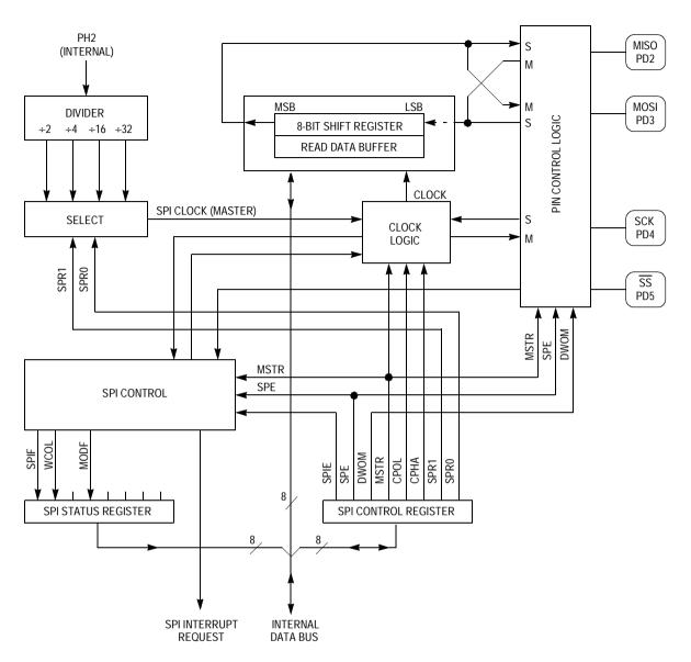
Figure 8-3. SPI System Block Diagram
