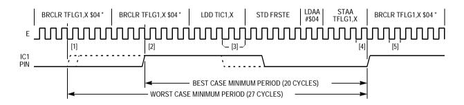
Figure 10-17. Timing Analysis for Example 10-1
