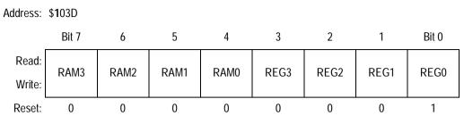
Figure 3-3. RAM and I/O Mapping Register (INIT)
