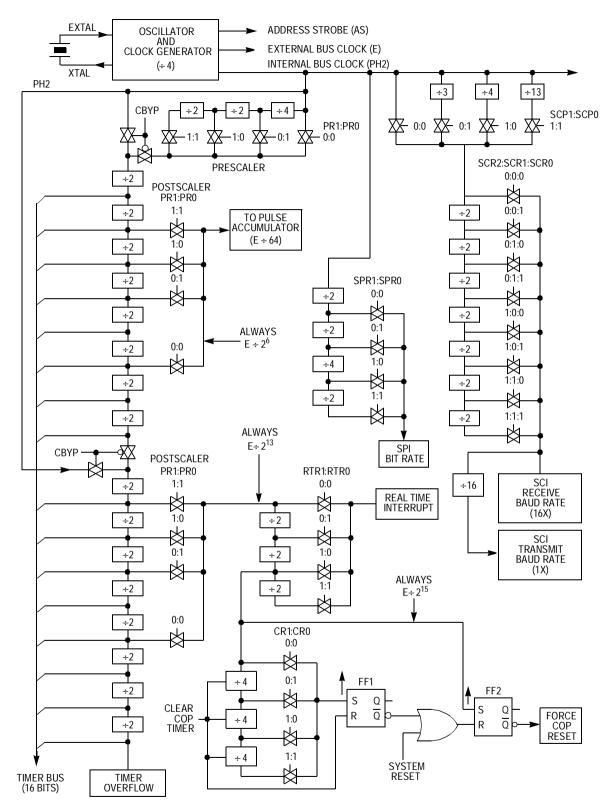
Figure 10-4. Major Clock Divider Chains in the MC68HC11A8
