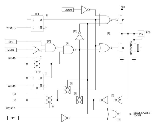
Figure 7-21. PD5 (SS) Pin Logic
