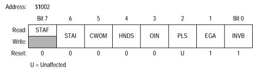
Figure 7-28. Parallel I/O Control Register (PIOC)
