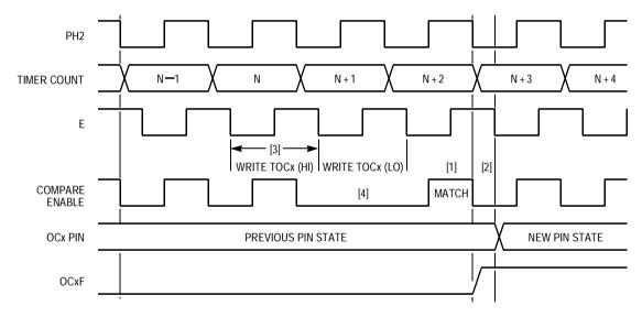
Figure 10-35. Output-Compare Timing Details
