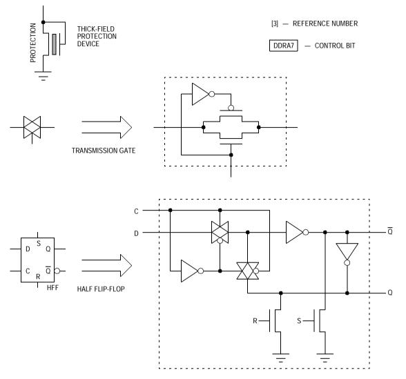
Figure 7-3. Special Symbols Used in Pin Logic Diagrams
