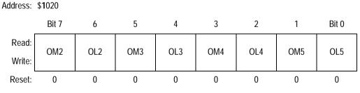
Figure 10-25. Timer Control Register 1 (TCTL1)
