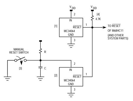
Figure 5-1. Typical External Reset Circuit
