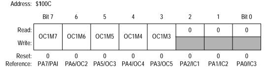
Figure 10-28. Output Compare 1 Mask Register (OC1M)
