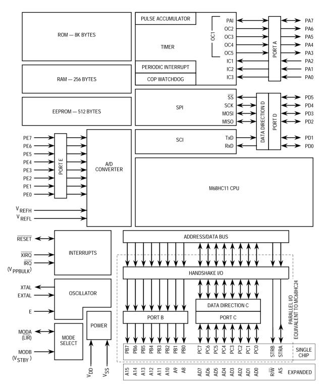
Figure 1-1. Block Diagram
