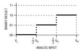
Without the extra 1-unit capacitor, each unit of capacitance corresponds to one-third the total rather than corresponding to the desired one-fourth. When the second 1-unit capacitor is added, the following circuit and transfer characteristics result:
