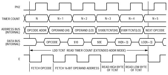
Figure 10-33. Timer Counter Read — Cycle-by-Cycle Analysis
