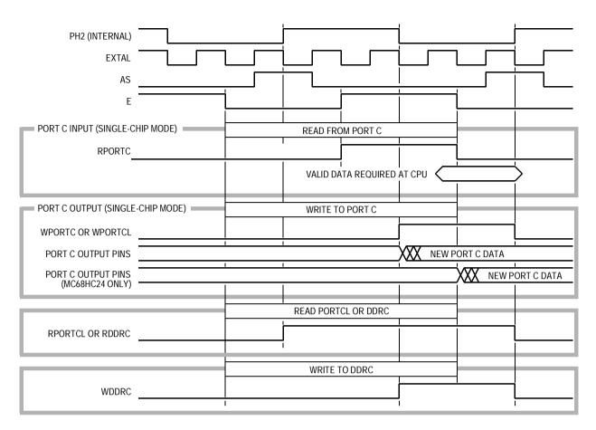
Figure 7-14. Idealized Port C Single-Chip Mode Timing
