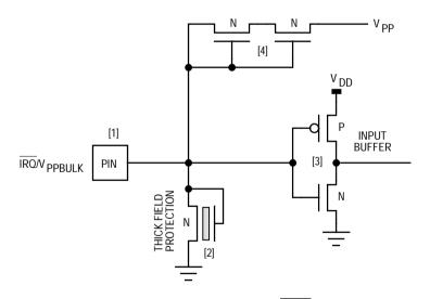
Figure 2-21. Internal Circuitry — IRQ/V<sub>PPBULK</sub> Pin
