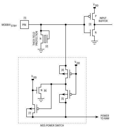
Figure 2-20. Internal Circuitry — MODB/V<sub>STBY</sub> Pin
