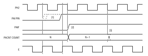
Figure 11-10. PAI Pin Edge-Detection Timing
