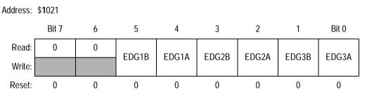
Figure 10-15. Timer Control Register (TCTL2)
