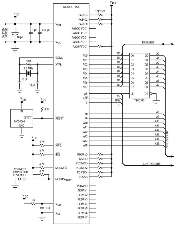
Figure 2-22. Basic Expanded Mode Connections (Sheet 1 of 2)
