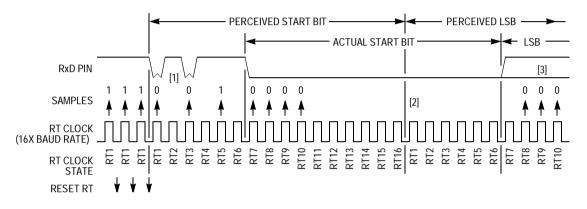
Figure 9-13. Start Bit — Noise Case Three
