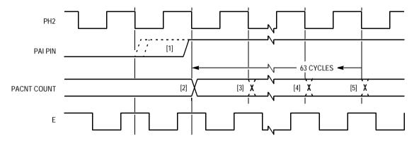
Figure 11-11. Pin Enable versus Counting (Gated Accumulation Mode)
