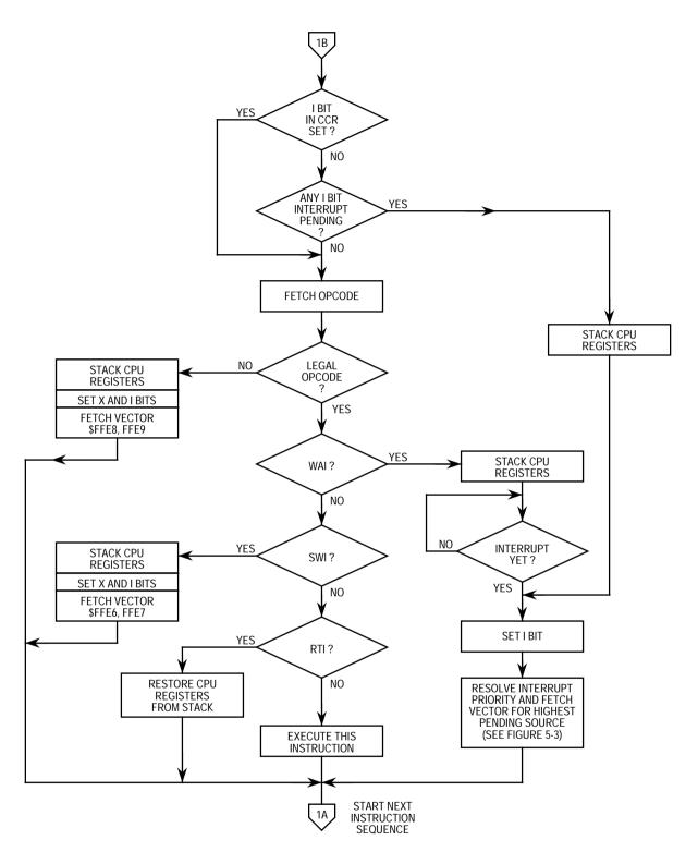
Figure 5-3. Processing Flow Out of Resets (Sheet 2 of 2)
