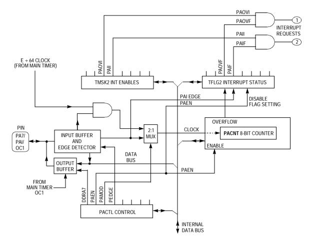
Figure 11-2. Block Diagram of Pulse Accumulator Subsystem
