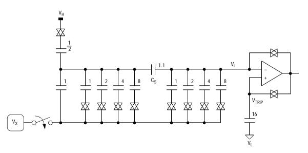
Figure 12-3. MC68HC11A8 A/D in Sample Mode
