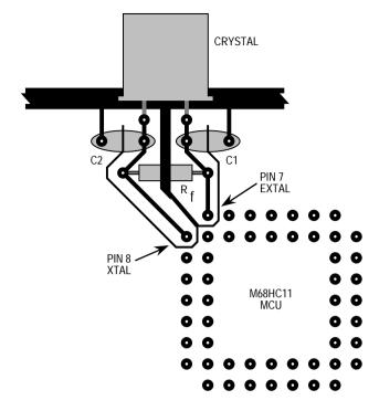
Figure 2-11. Crystal Layout Example
