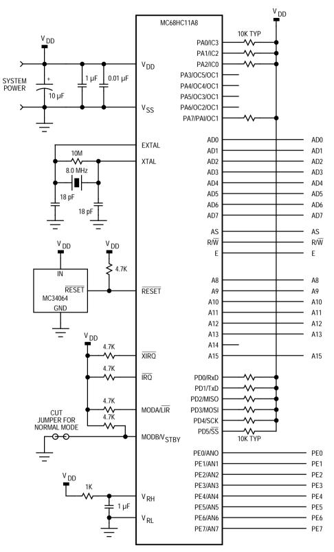
Figure 3-8. Schematic for Figure 3-9 (Sheet 1 of 2)
