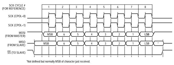
Figure 8-1. CPHA Equals Zero SPI Transfer Format
