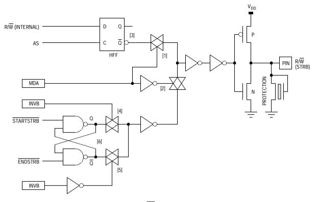
Figure 7-10. R/W (STRB) Pin Logic
