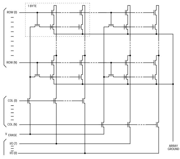
Figure 4-3. Condensed Schematic of EEPROM Array
