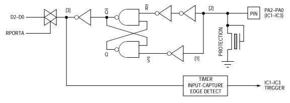
Figure 7-4. PA2–PA0 (IC3–IC1) Pin Logic
