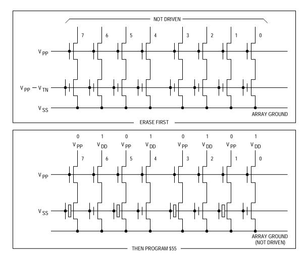
Figure 4-9. Erase-Before-Write Programming Method
