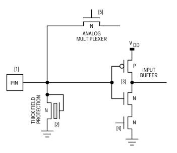
Figure 2-16. Internal Circuitry — Analog Input-Only Pin
