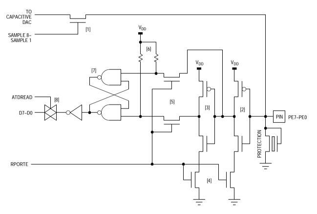
Figure 7-23. Port E Pin Logic
