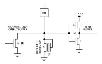
Figure 2-18. Internal Circuitry — Input/Open-Drain-Output Pin
