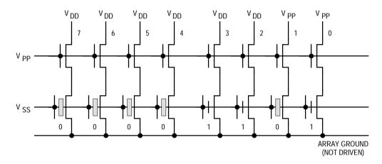
Figure 4-12. Composite Programming Method
