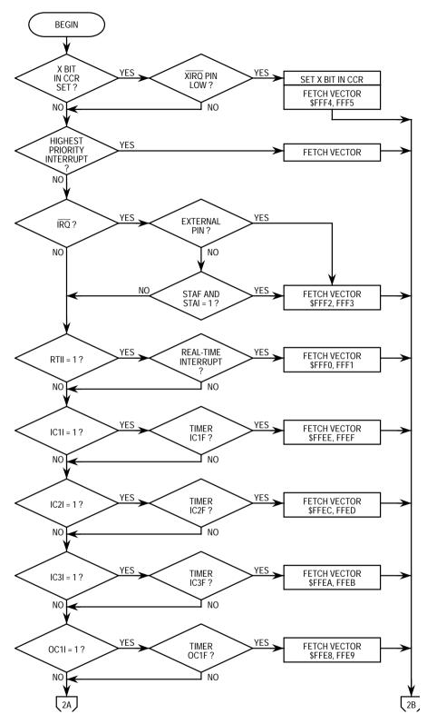
Figure 5-4. Interrupt Priority Resolution (Sheet 1 of 2)
