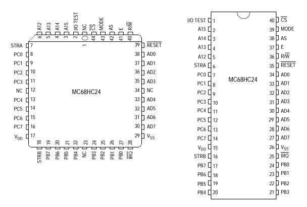
Figure 2-6. MC68HC24 Pin Assignments
