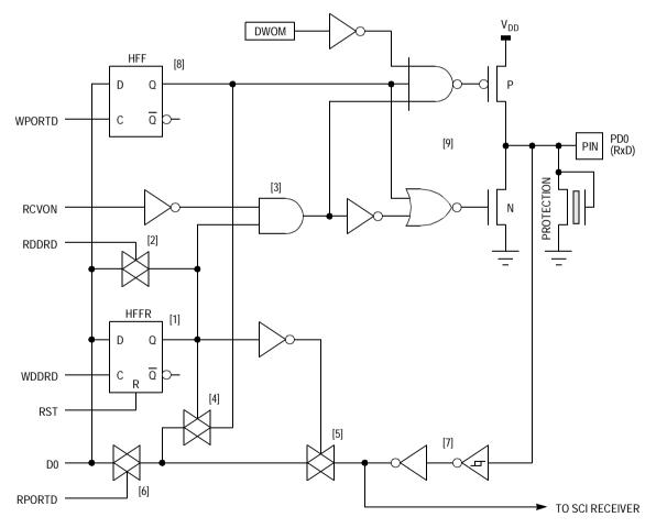
Figure 7-16. PD0 (RxD) Pin Logic
