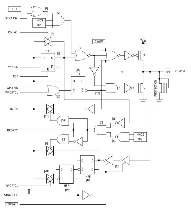
Figure 7-13. Port C Single-Chip Mode Pin Logic
