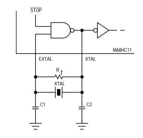
Figure 2-9. High-Frequency Crystal Connections
