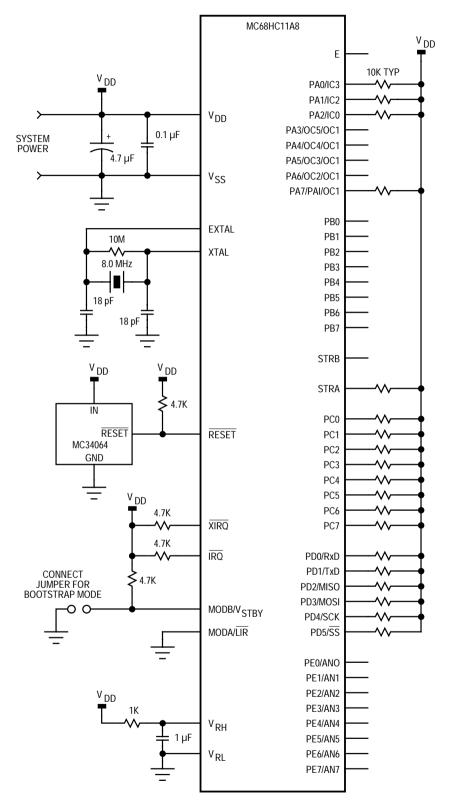
Figure 2-23. Basic Single-Chip Mode Connections
