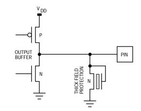
Figure 2-19. Internal Circuitry — Output-Only Pin
