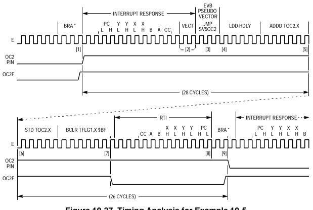
Figure 10-27. Timing Analysis for Example 10-5
