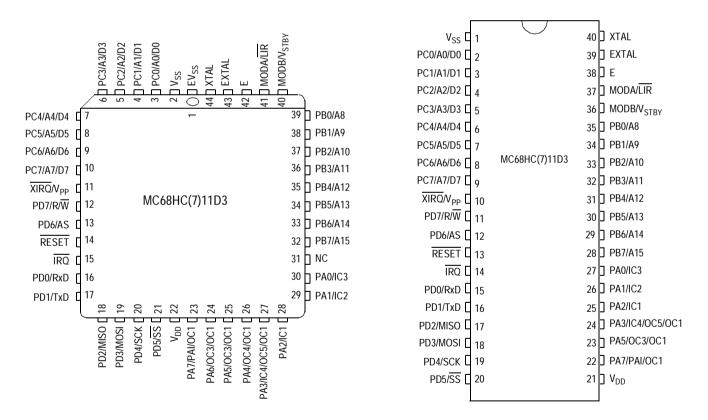
Figure 2-2. MC68HC11D3/711D3 Pin Assignments
