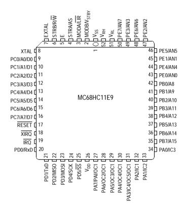
Figure 2-3. MC68HC11E9/711E9 Pin Assignments (52-Pin PLCC)
