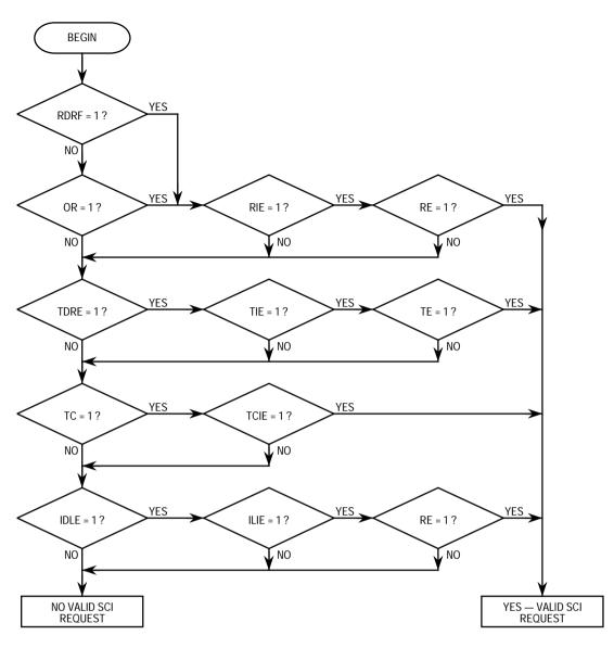
Figure 5-5. Interrupt Source Resolution within SCI
