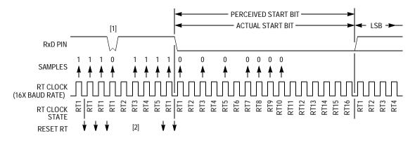
Figure 9-11. Start Bit — Noise Case One
