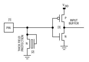
Figure 2-15. Internal Circuitry — Digital Input-Only Pin
