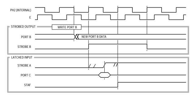
Figure 7-25. Idealized Timing for Simple Strobe Operations
