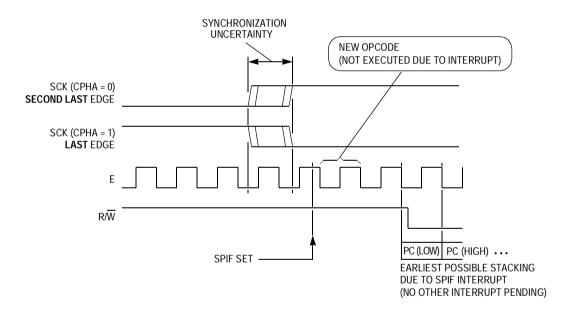
Figure 8-9. Transfer Ending for an SPI Slave
