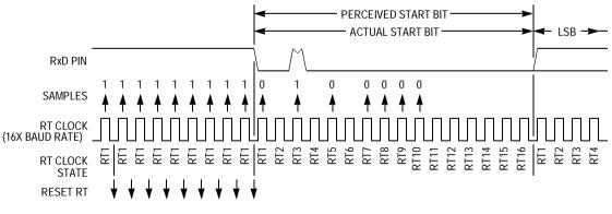
Figure 9-14. Start Bit — Noise Case Four
