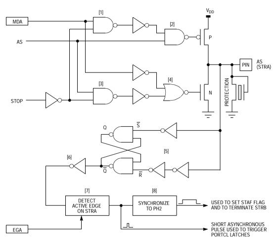
Figure 7-15. AS (STRA) Pin Logic
