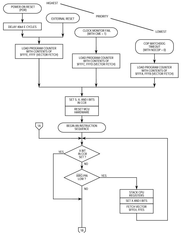
Figure 5-3. Processing Flow Out of Resets (Sheet 1 of 2)
