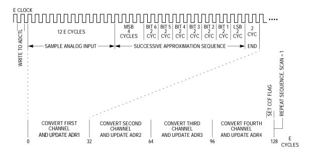
Figure 12-5. Timing Diagram for a Sequence of Four A/D Conversions
