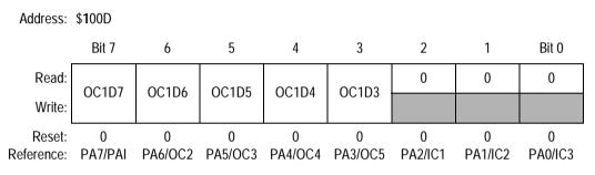
Figure 10-29. Output Compare 1 Data Register (OC1D)
