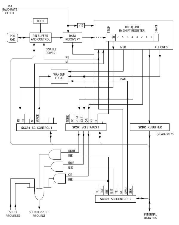
Figure 9-2. SCI Receiver Block Diagram
