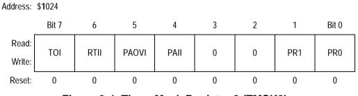
Figure 3-4. Timer Mask Register 2 (TMSK2)
