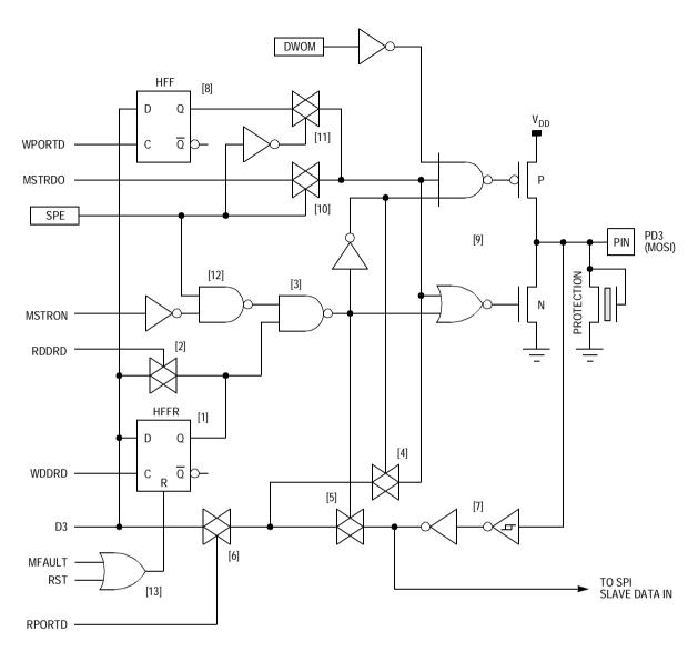
Figure 7-19. PD3 (MOSI) Pin Logic
