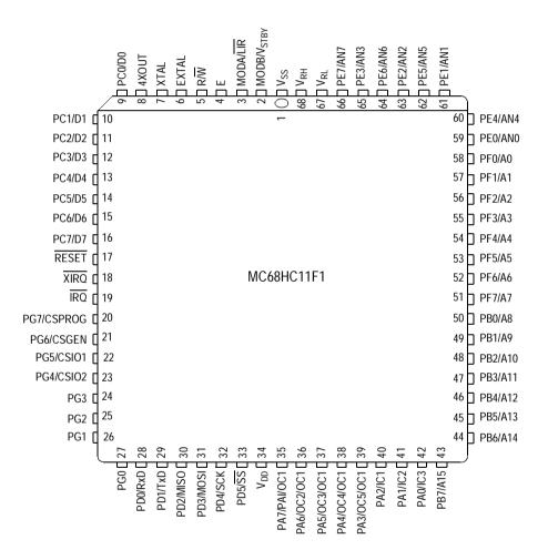
Figure 2-5. MC68HC11F1 Pin Assignments (68-Pin PLCC)
