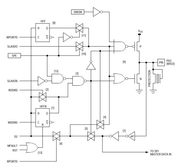
Figure 7-18. PD2 (MISO) Pin Logic
