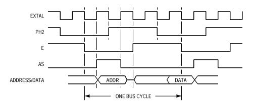
Figure 10-3. Timing Summary for Oscillator Divider Signals
