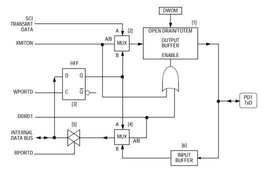
Figure 9-9. TxD Pin Logic Block Diagram
