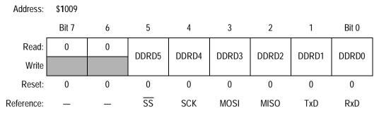
Figure 8-4. Port D Data Direction Register (DDRD)
