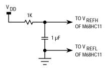
Figure 2-13. Low-Pass Filter for A/D Reference Pins
