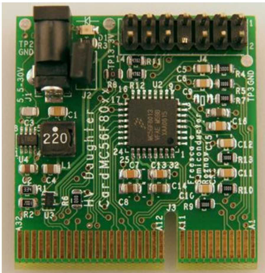
Figure 2-15. MC56F80xx high voltage daughter board card
