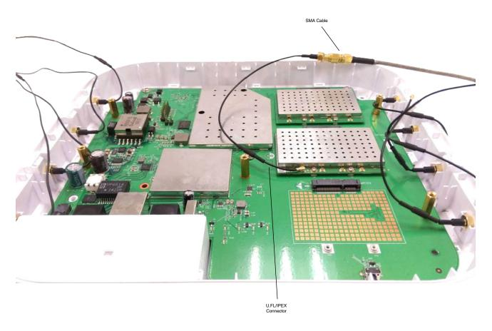
Figure 6. T1023 board cables connected with the antennas
