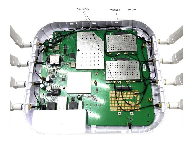
Figure 3. Top view of T1023 board
