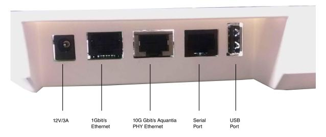
Figure 2. Front view of T1023 board
