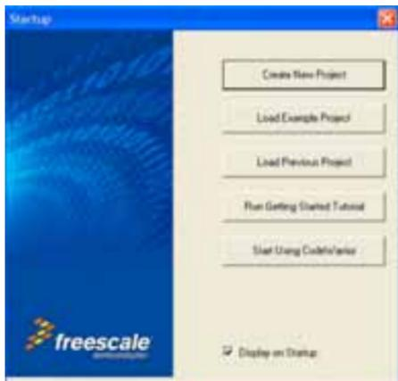
Figure 3. Showing startup dialog that appears when you start CodeWarrior. You can choose to Load Example Project from other various S08 devices.
