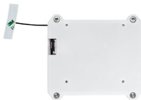
Figure 3: Bottom view — NavQPlus with case
