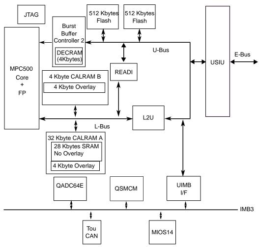
Figure 1. MPC535 Block Diagram
