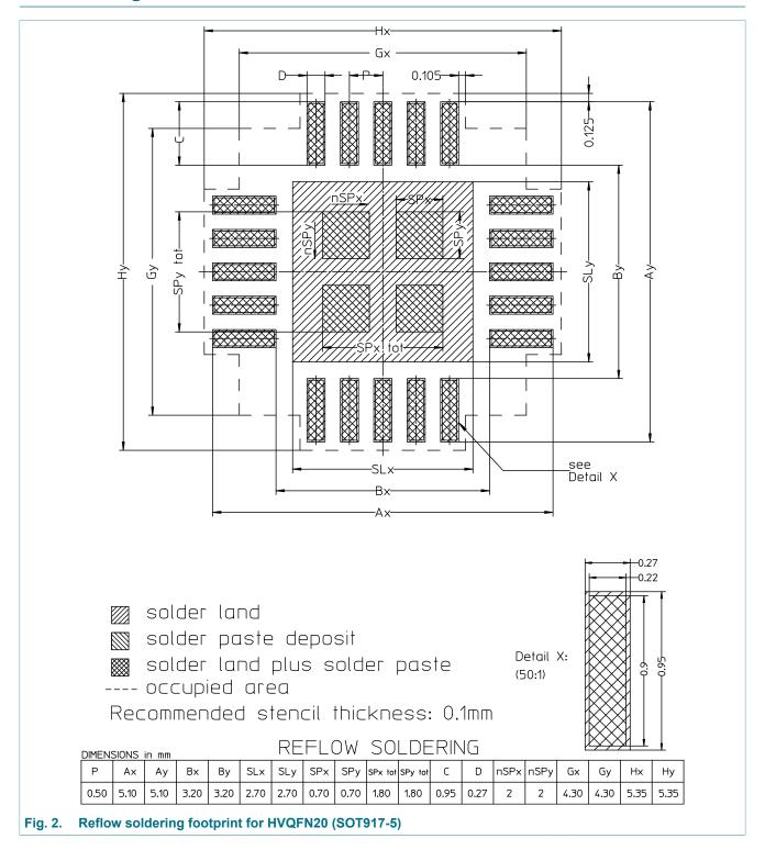
HVQFN20, plastic thermal enchanced very thin quad flat package; no leads; 20 terminals; 4 mm x 4 mm 0.85 mm body
