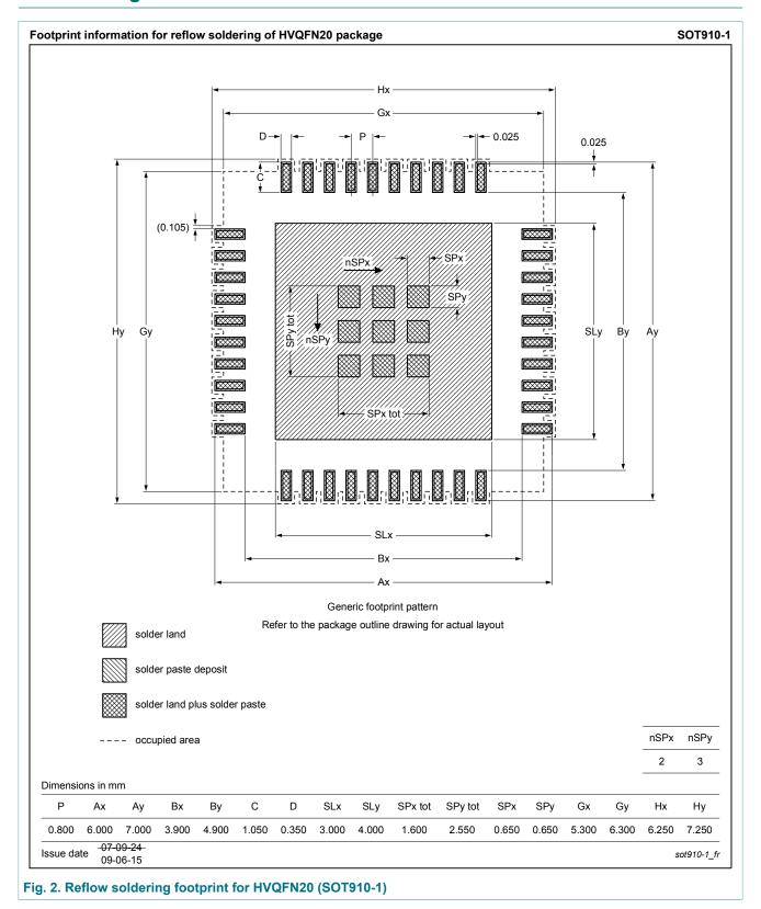
plastic thermal enhanced very thin quad flat package; no leads; 20 terminals; body 6 x 5 x 0.85 mm
