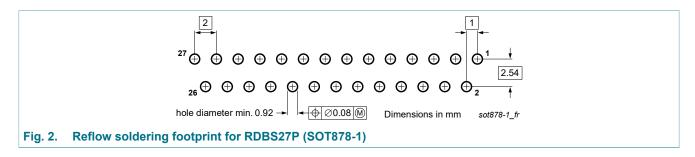
plastic rectangular-DIL-bent-SIL (reverse bent) power package; 27 leads, (row spacing 2.54 mm)
