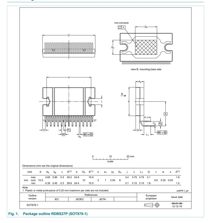
plastic rectangular-DIL-bent-SIL (reverse bent) power package; 27 leads, (row spacing 2.54 mm)
