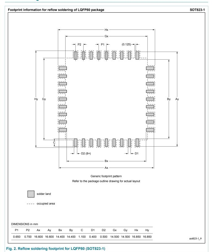
plastic low profile quad flat package; 80 leads; body 14 x 14 x 1.4 mm
