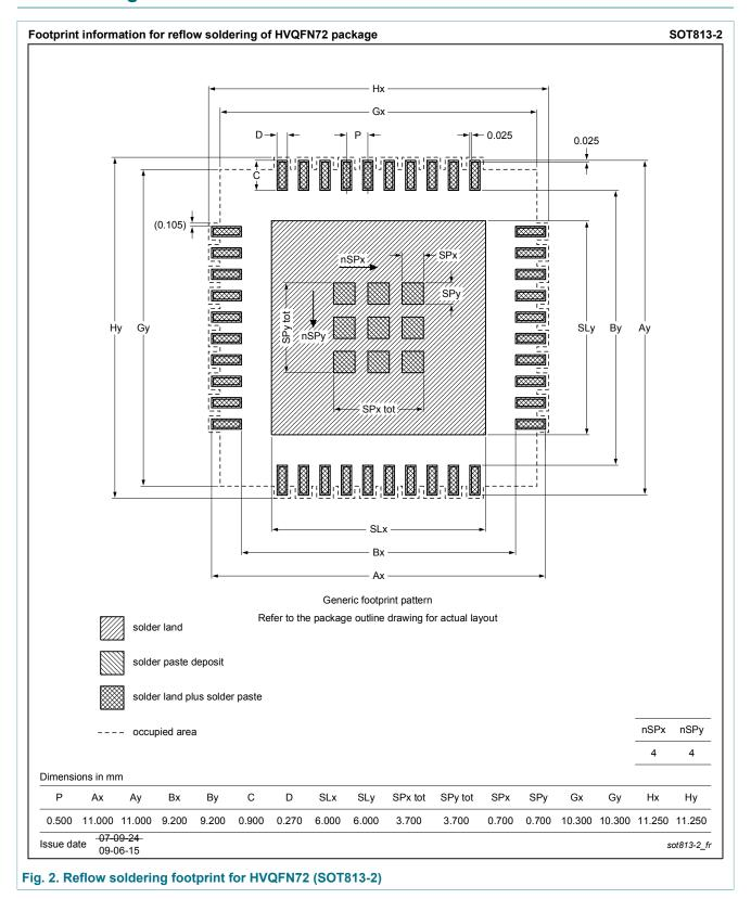
plastic thermal enhanced very thin quad flat package; no leads; 72 terminals
