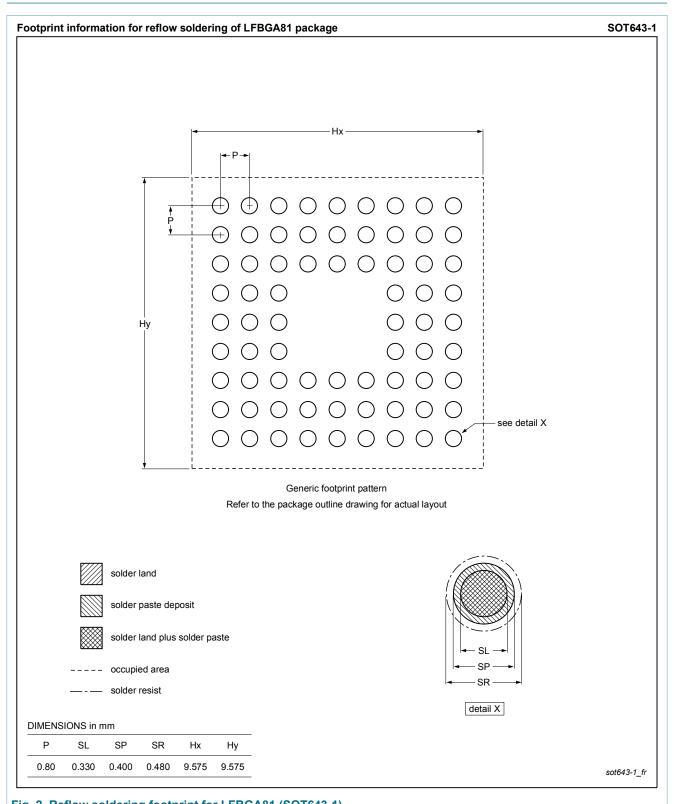
Fig. 2. Reflow soldering footprint for LFBGA81 (SOT643-1)
