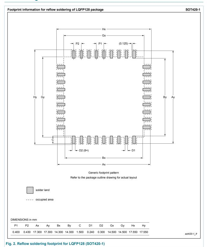
plastic low profile quad flat package; 128 leads; body 14 x 14 x 1.4 mm
