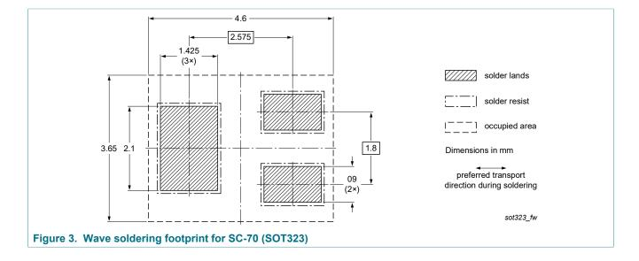
plastic, surface-mounted package; 3 leads; 1.3 mm pitch; 2 mm x 1.25 mm x 0.95 mm body
