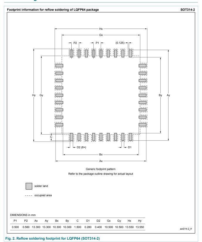
plastic low profile quad flat package; 64 leads; body 10 x 10 x 1.4 mm
