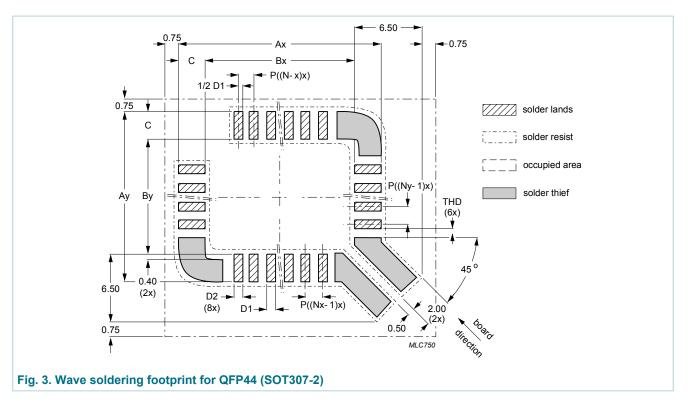
plastic quad flat package; 44 leads (lead length 1.3 mm); body 10 x 10 x 1.75 mm
