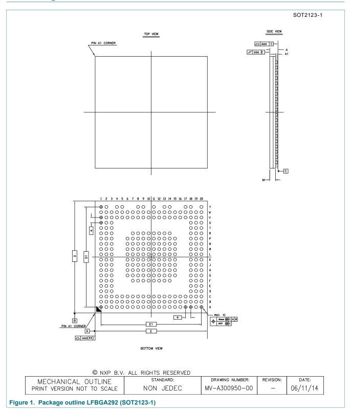
LFBGA292, low profile, fine-pitch ball grid array package, 292 terminals, 0.8 mm pitch, 17 mm x 17 mm x 1.24 mm body
