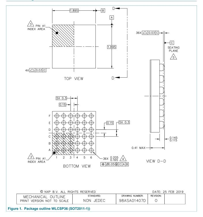
WLCSP36, wafer level chip scale package, 36 terminals, 0.3 mm pitch, 1.895 mm x 1.895 mm x 0.38 mm body (backside coating included)
