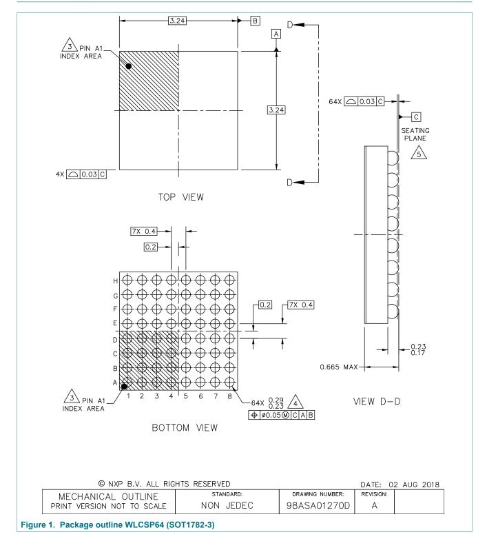
WLCSP64, wafer level chip-scale package; 64 bumps; 3.24 mm x 3.24 mm x 0.625 mm body (backside coating included)
