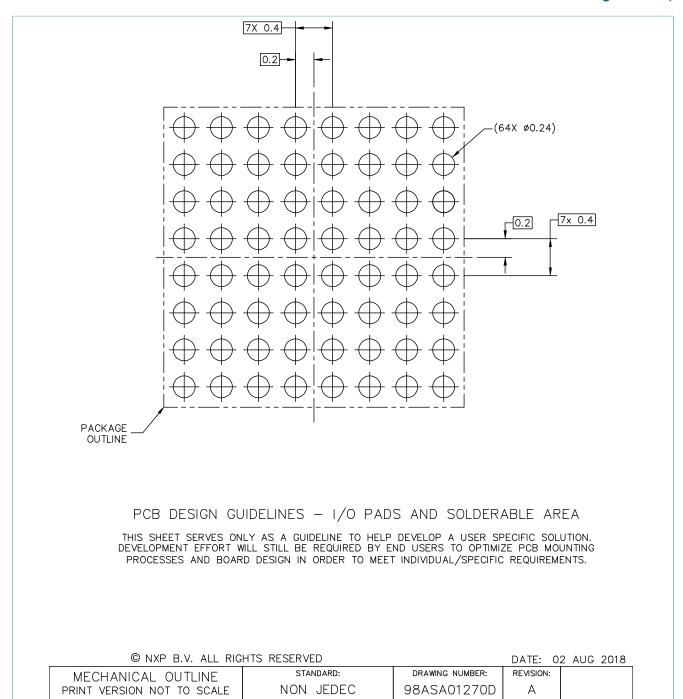
Figure 4. Reflow soldering footprint part2 for WLCSP64 (SOT1782-3)
