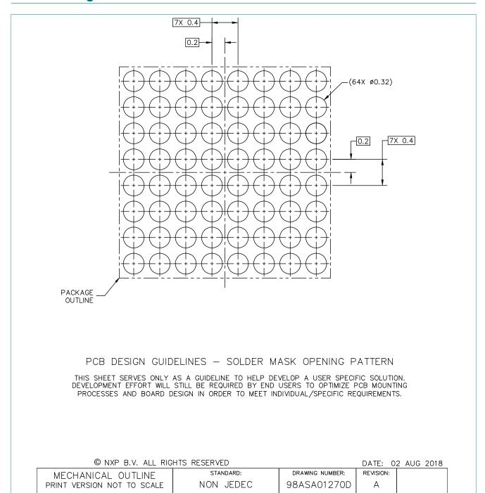
Figure 3. Reflow soldering footprint part1 for WLCSP64 (SOT1782-3)
