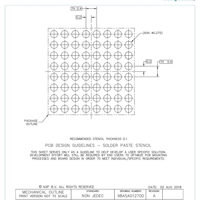
Figure 5. Reflow soldering footprint part3 for WLCSP64 (SOT1782-3)
